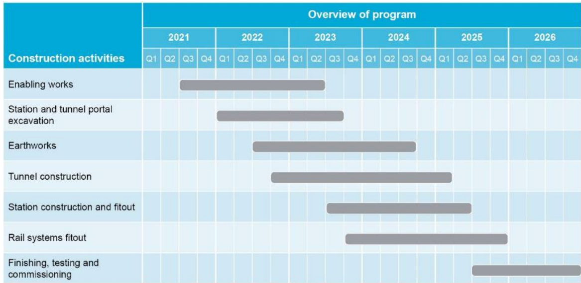
Figure 1-2 Indicative main construction program
