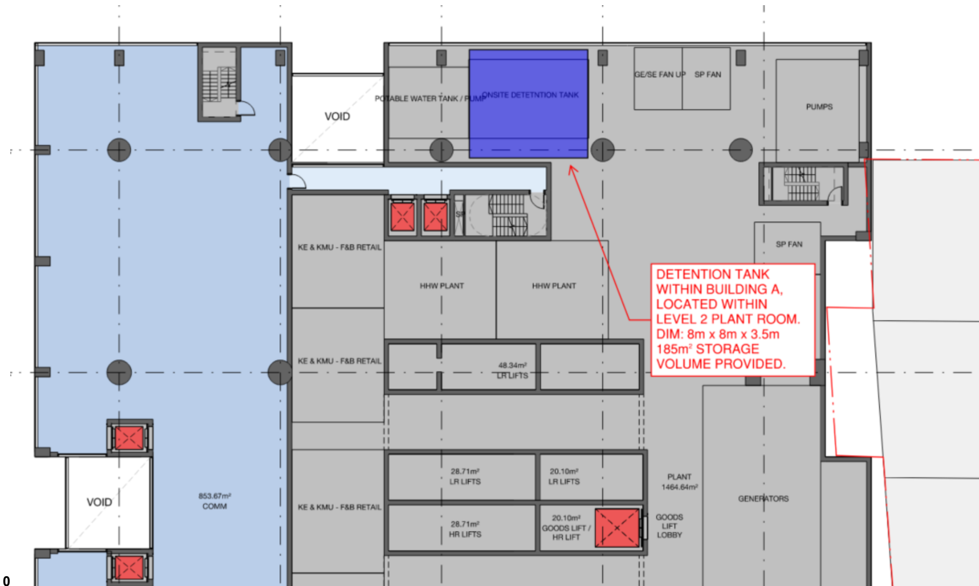
Figure 5 Building A DOSD Tank Location
