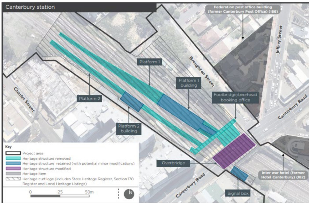
Figure 1 Location of Footbridge within Canterbury Station
