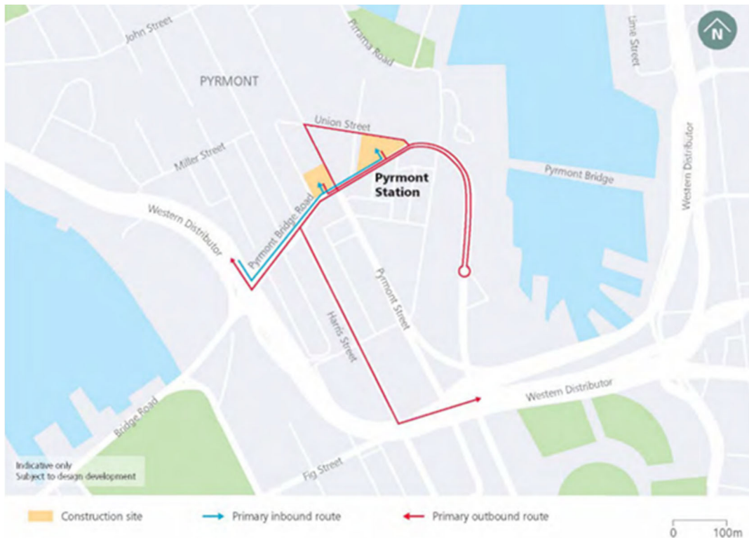
Figure 6-1 CSSI construction haulage routes, Pyrmont Station
