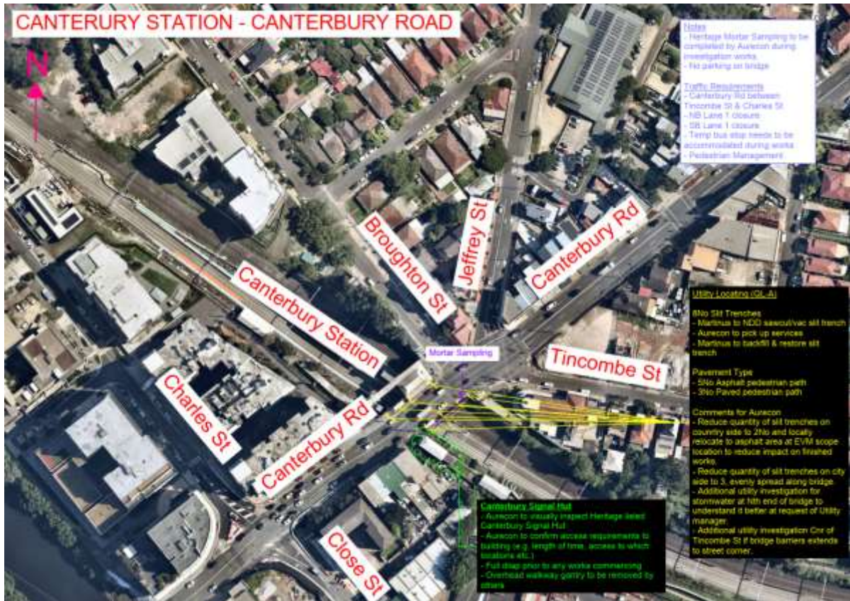
Figure 7: Site Investigation Plan (Source: Arch Artifex/ Martinus)
