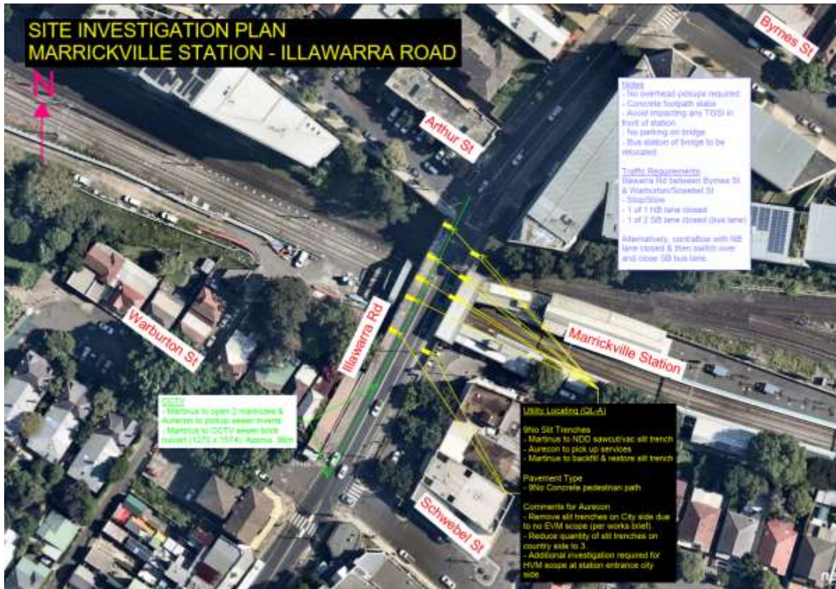
Figure 3: Site Investigation Plan (Source: Arch Artifex/ Martinus)
