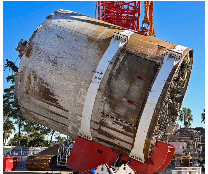
You spin me right round – TBM Betty's gripper shield, a cover of the internal mechanisms of the machine, retrieved and rotated ahead of its transportation back to Clyde.
