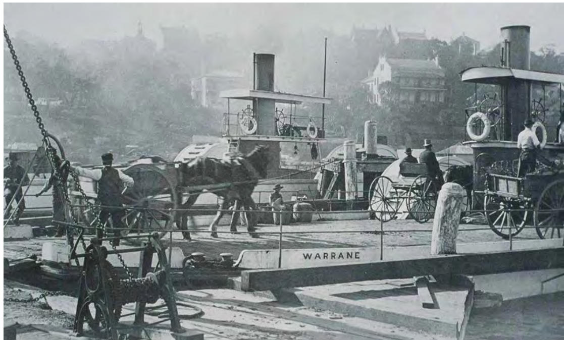
Figure 13: Loading the vehicular horse ferry at Blues Point ferry wharf, City of Sydney Archives A-00076337, n.d. This vessel was in service between 1883 and 1921, superseded by larger ferries capable of carrying the heavier weight of motorised vehicles.
