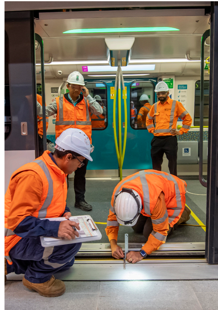
Train to platform measurement checks
