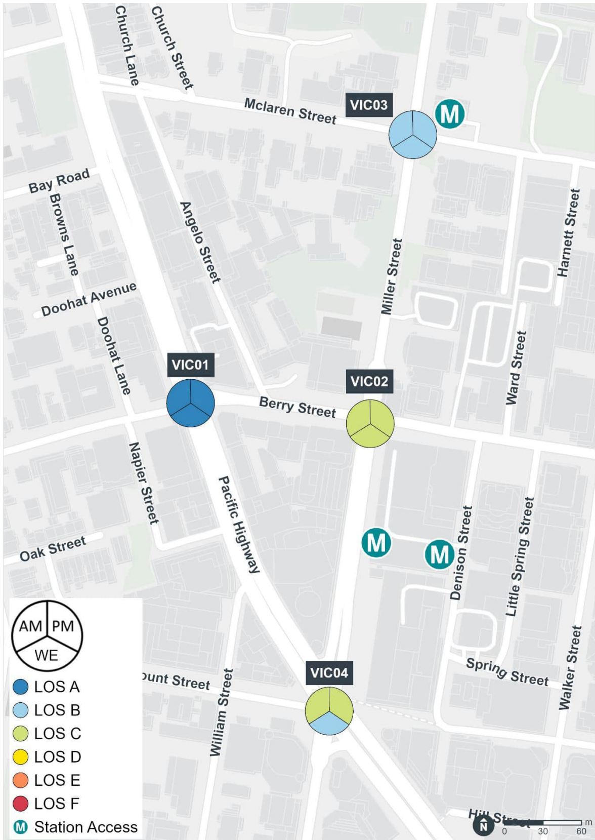
Figure 5-22 Block 3 – Victoria Cross Station intersection performance summary
