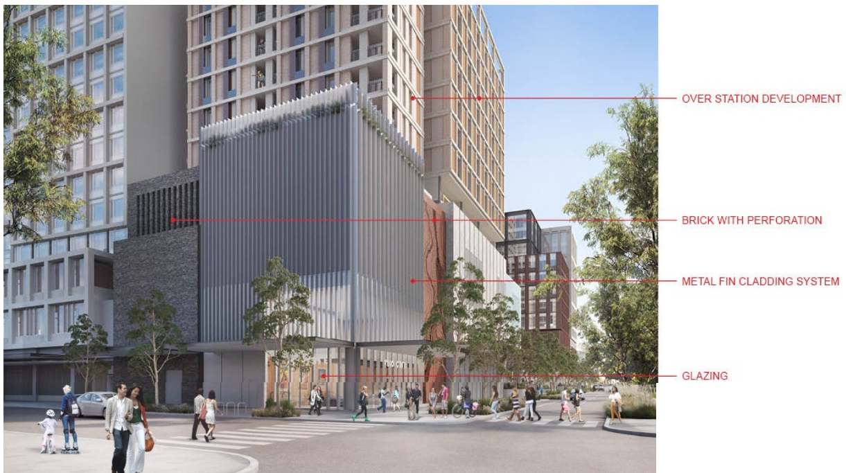
Figure 6.1.2.4: An artist’s impression of the Wellington Street southern station building façade finishes
