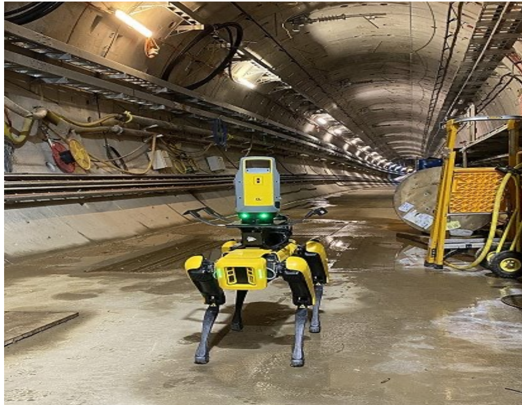
Trialling an autonomous asset inspection robot.
