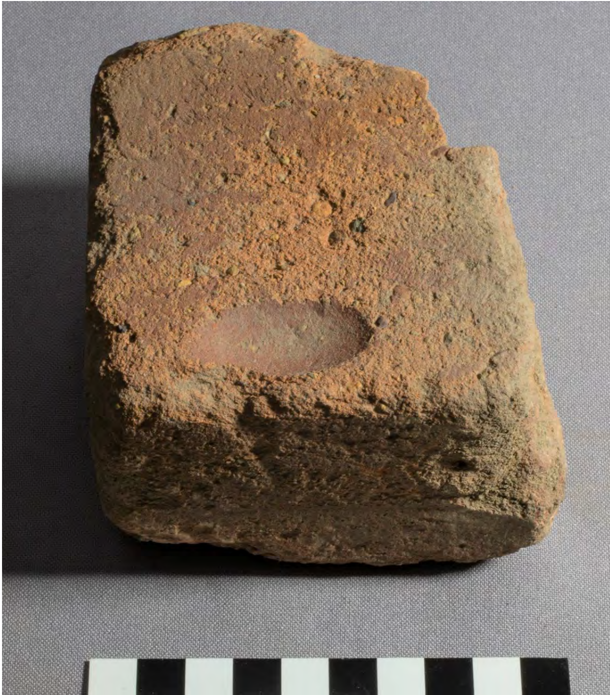
Figure 4.5: O29/#15003, an unfroged dry-pressed brick with a thumb tally mark which has a red slip. 100mm scale. IMG_2929. R. Workman.
