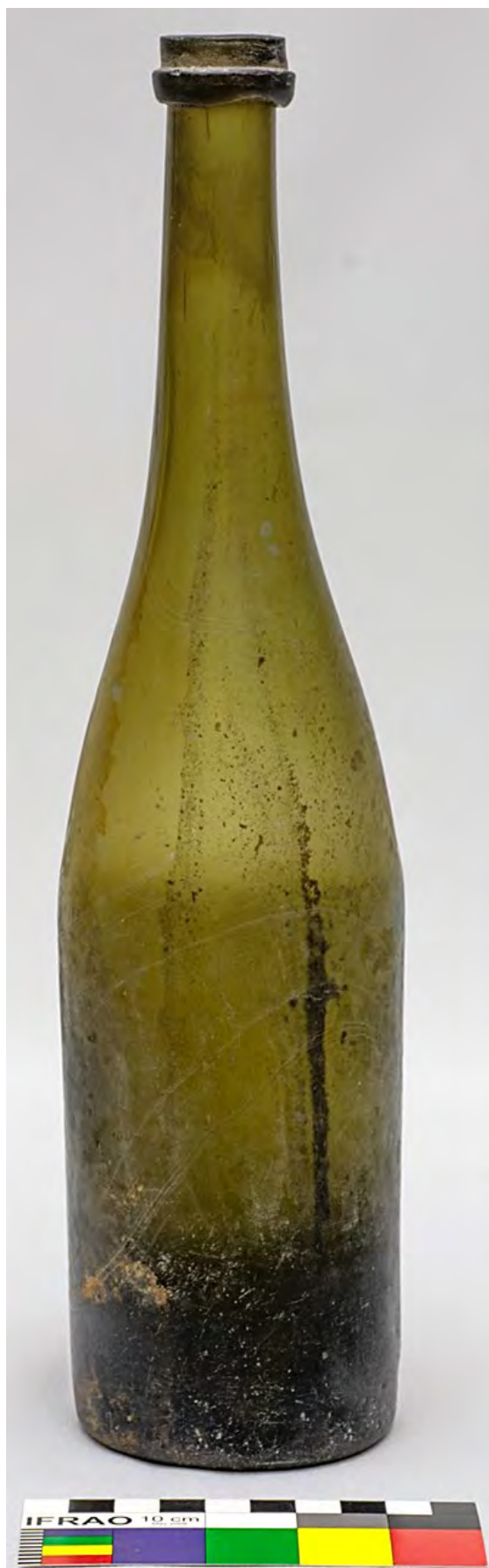
Figure 2.6: Dip-moulded conical push up champagne bottle with sand pontil scar 149/#366. 100mm scale. DSC_1753. R. Workman.
