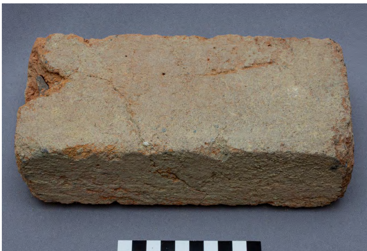
Figure 4.3: 108/#15006, a sandstock flat with the horizontal hack marks visible on the strikeface and crumbly buff shell sand mortar. 100mm scale. IMG_3919. R. Workman.
