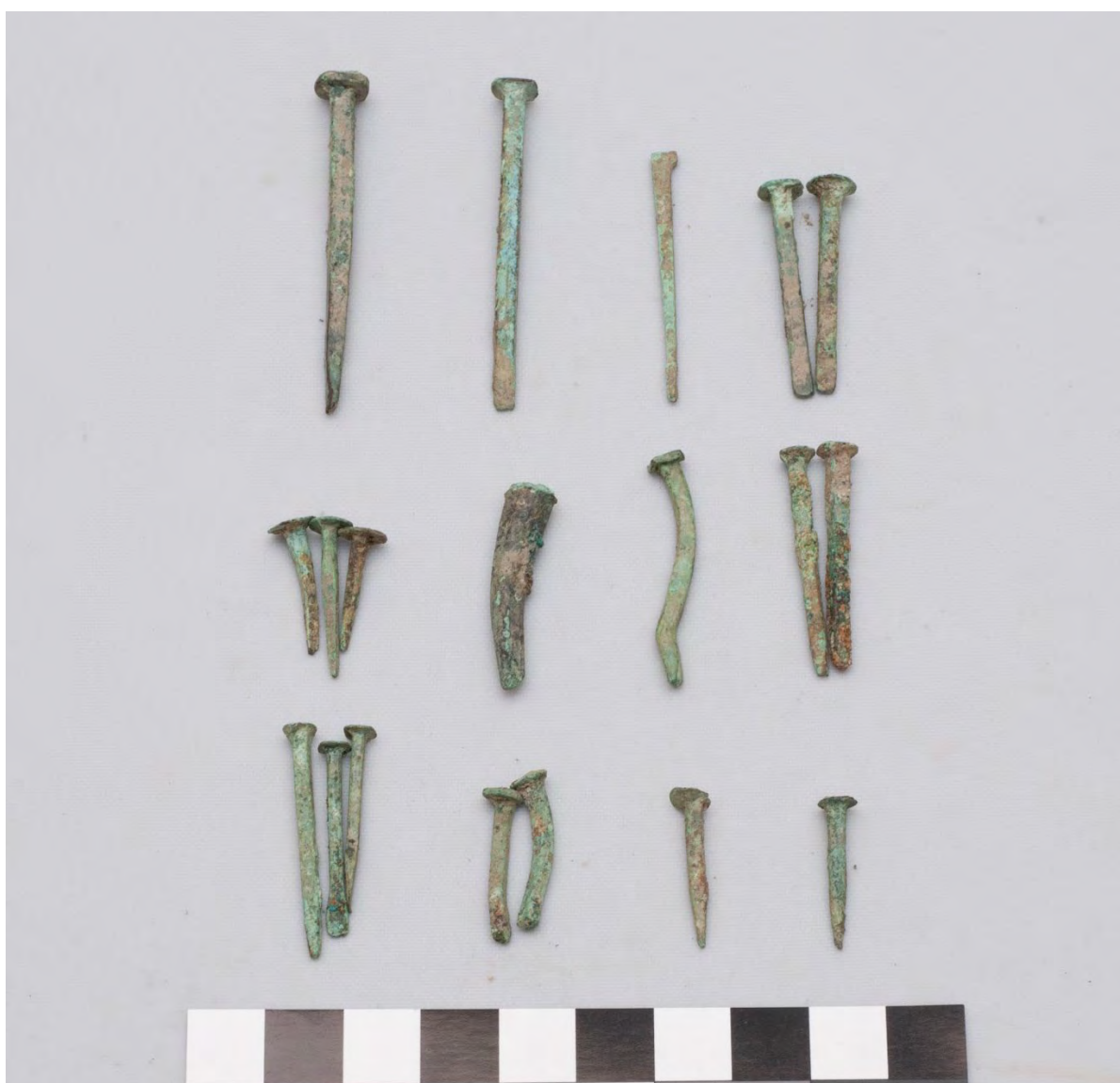
Figure 3.8: Copper alloy household/transport and transport nails from context 124. (l-r) Top row: WD sq nails #2149 and #2148, Cut Brad nail #2146, WD sq nails #2150. Second row: small tacks #2160, HF nail #2147, Wd sq nails #2162 and #2154. Bottom row: WD sq nails and tacks #2153, #2161, #2159, #2158. 100mm scale. IMG_5438. R. Workman.
