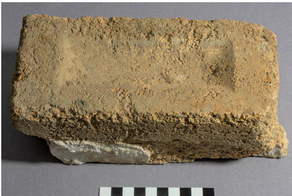
Figure 4.4: 200/#15021, a typical example of the inverted-hip frogged dry-pressed bricks catalogued from the site. 100mm scale. IMG_3925. R. Workman.
