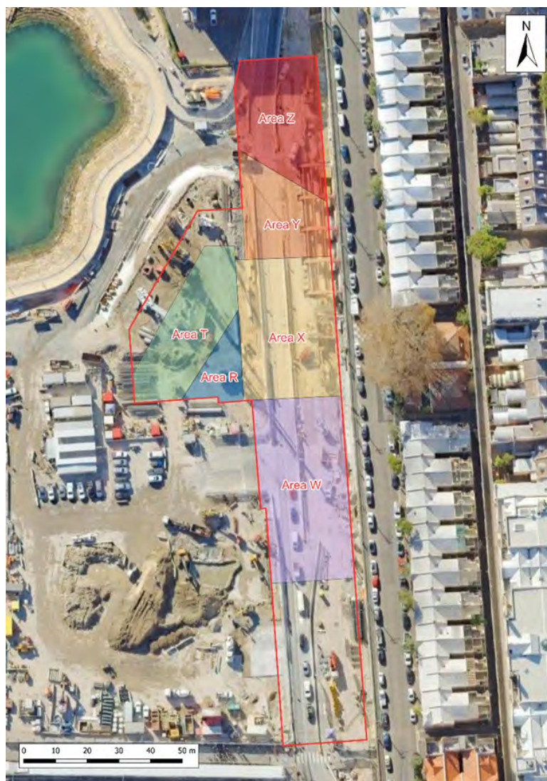
Figure 1.1: Location plan showing the Barangaroo Station site outlined in red and the excavation areas are shaded. Google Maps.
