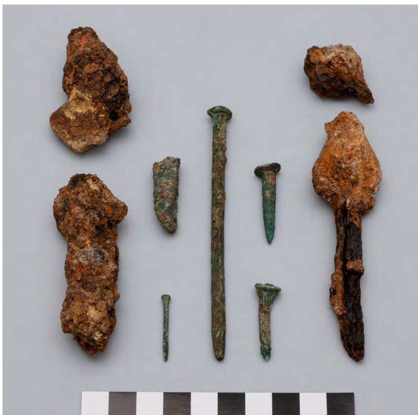
Figure 3.5: Iron and copper alloy nails from contexts associated with Dibbs wharf (O31, O72, O63, O58). Top to bottom, first column: hand-forged iron nail O63/#2052. Second column: copper alloy spike #2056, WD sq tack O58/#2049. Middle: WD sq boat nail O31/#2039. Fourth column: sheathing nails O72/#2055, O72/#2057. Last column: unidentified iron tool O63/#2051. 100mm scale. IMG_5439. Russell Workman.
