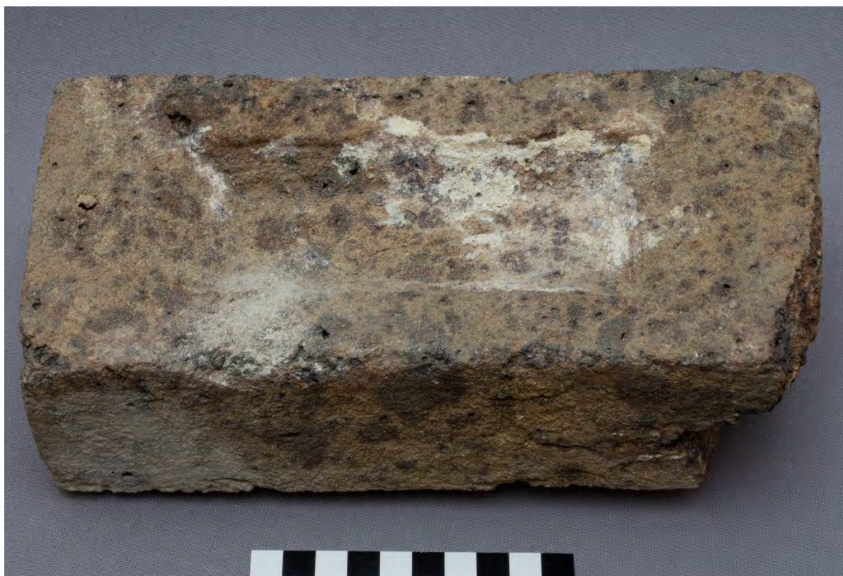
Figure 4.2: 170/#15019, a sandstock brick with a rectangular frog dating from 1850 to 1900. 100mm scale. IMG_3917. R. Workman.
