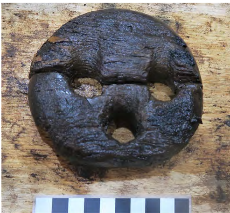
Figure 3.18: Element (065). Circular dead eye. Note this has been cut with the grain of the wood opposing the rope which caused the split. Scale 100mm. Img_2262.
