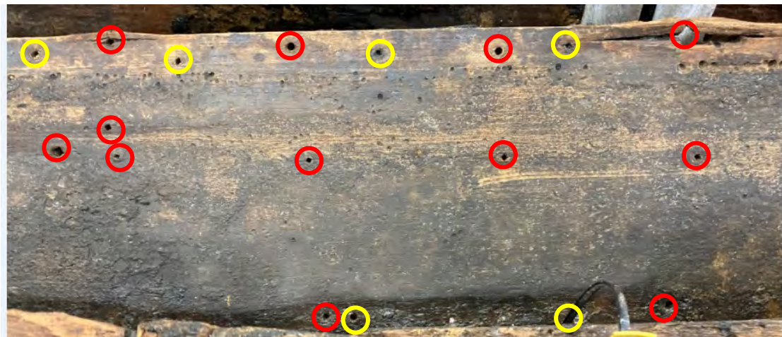
Figure 4.80: Plank [313 S-I-S2-A] possible fastener pattern. Red circles for plank-to-plank, yellow for frame-to-plank. External side of plank may show blind holes from secondary outer planking. (Source: Benjamin Wharton 2020).
