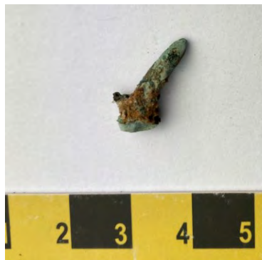
Figure 4.14: Copper alloy fastener from garboard shelf [539]. (Source: Benjamin Wharton 2020).
