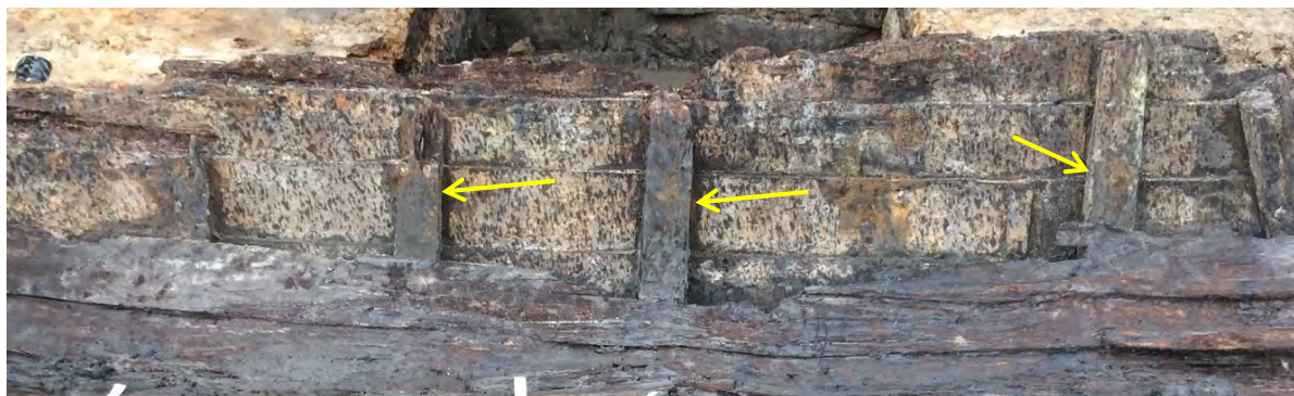
Figure 4.104: Starboard side ceiling planks futtock frames. Iron staining evident on frames suggest possibility of ceiling planks existing higher up the topside, or where a rising was fastened to. (Source: AMBS).
