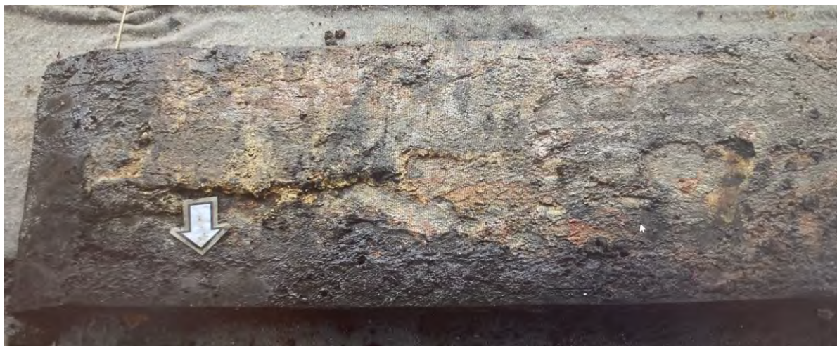
Figure 5.5 : Remains of pitch visible under chunam on outer side of inner planking [486]
