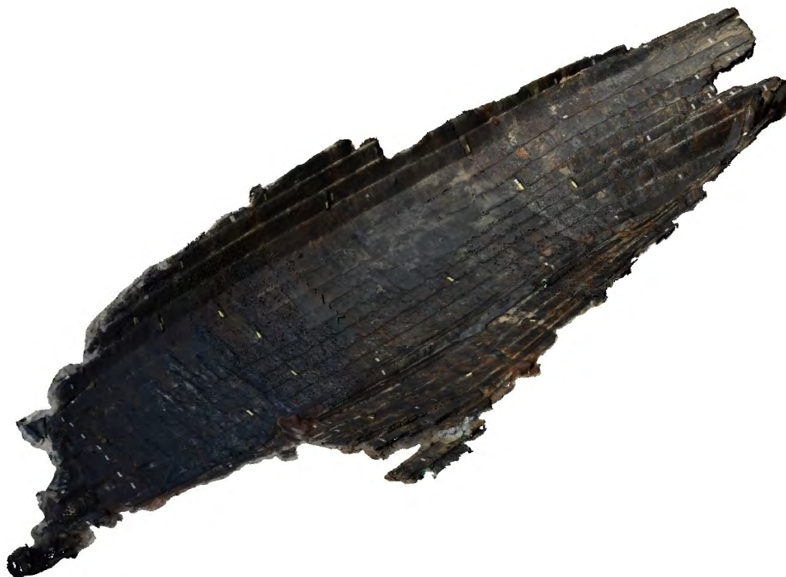
Figure 4.45: Isometric view of inner hull planking after frames removed. Chine visible between the eighth and ninth strakes being the intermediate bilge area between the bottom and topside strakes of the hull. Bow bottom left. (Source: photogrammetry recording and model by Guy Hazel 2018).
