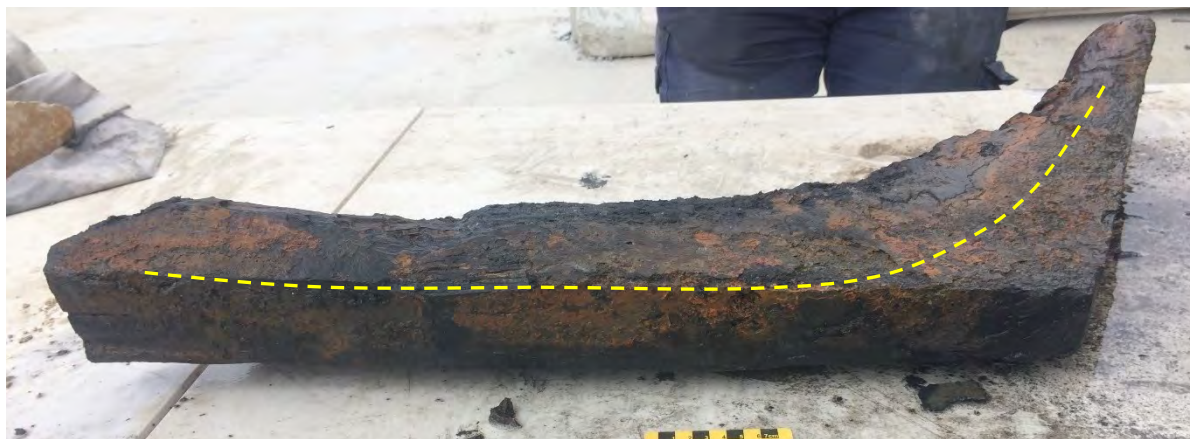
Figure 4.25: Underside face of stern knee that connects to the top face keel line. Note the taper in plain view reducing abaft. Also note the bearding line shown dashed which in cross section tapers also down from this line. (Source: AMBS).
