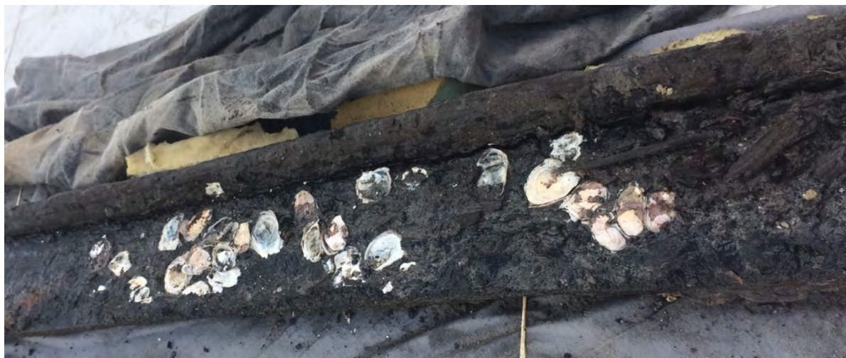
Figure 4.121: Pitch embedded with shells on garboard shelf [543]. (Source: AMBS).
