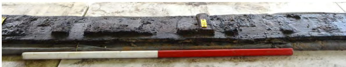
Figure 4.120: Pitch on internal side of Plank [495 S-I-S2-F]. Internally applied between framing as thick as the planking itself. (Source: Casey & Lowe).
