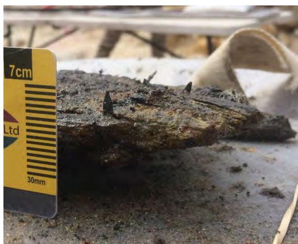
Figure 4.73: Tips of copper fasteners in situ. Aft-end of plank [464, SO-S09-A]. (Source: AMBS).
