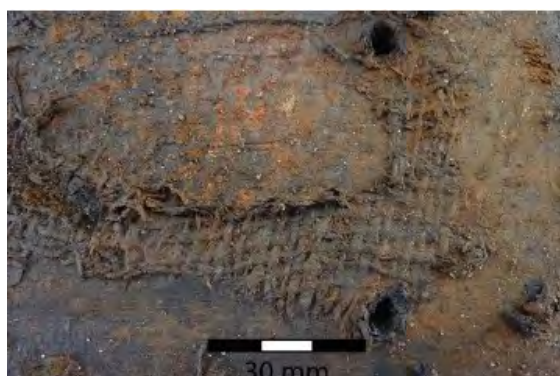
Figure 5.35: Textile used as caulking on the scarp between planks in the Mönchgut 92 wreck. (Source: Fiedler, K., 2016)
