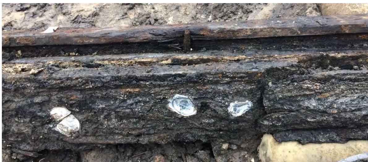
Figure 4.16: External surface of the starboard garboard shelf boards [539] and [540], view of starboard side. Showing scarf joint, heavy application of pitch, and the accumulation of shells. (Source: Benjamin Wharton 2018).
