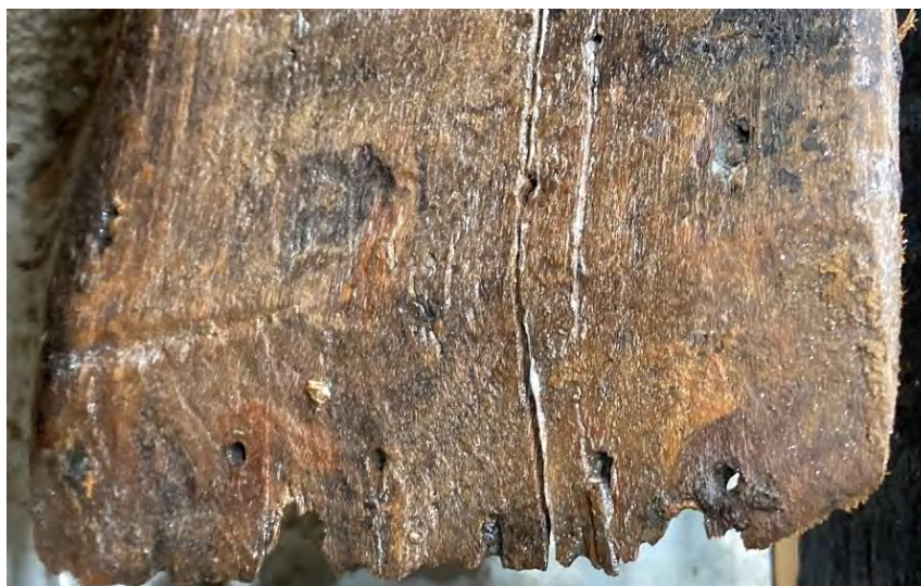
Figure 4.68: Scarf showing rings of grain having been plain sawn [517 SI-S5-M]. (Source: Benjamin Wharton 2021).
