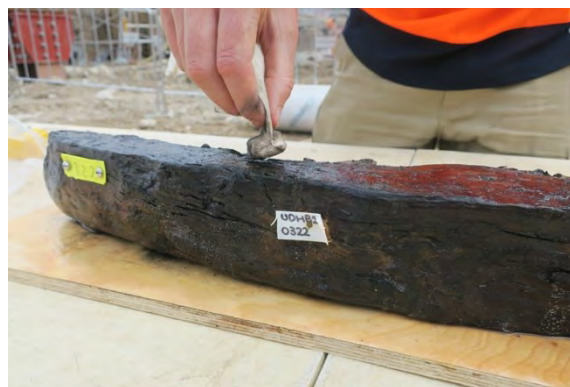
Figure 2.80: Detecting iron with earth magnet.
