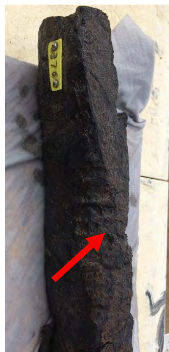
Figure 4.95: Branch collars (red arrow) on futtock frame [362] FT-3. (Source: AMBS).
