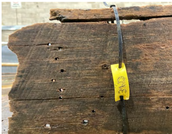
Figure 4.66: Pitsaw marks on plank [310] P-O-S2-A. Some cut lines with a pit saw sometimes appear curved from when sawyers changed stance or grip. (Source: Benjamin Wharton 2020).
