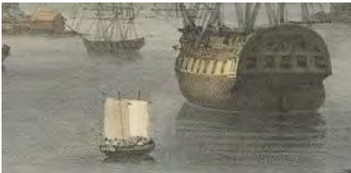
Figure 5.27: Detail of illustration 'Coming to an Anchor off Sydney Cove'. Lugsail ketch sail configuration with two masts.
