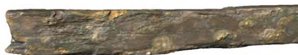
Figure 5.2 : View of aft end, starboard side of rider keel [551]. Note the worn underside but smooth topside. This upper side was in contact with the underside of the keel. (3D scans supplied by SWF)
