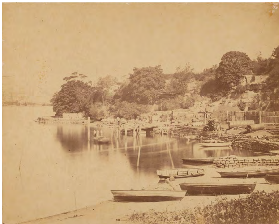
Figure 5.45: Blues Point, North Shore 1850s. Note the clinker-built boats with hard chine drawn up onto the beach. UDHB1 had a similar shaped hull.
