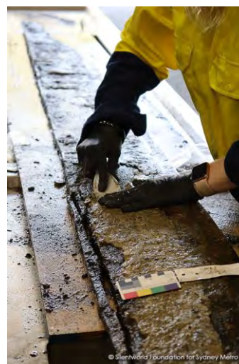
Figure 15: White material, possibly for anti-fouling, being removed during the conservation process. Source: Silentworld Foundation.
