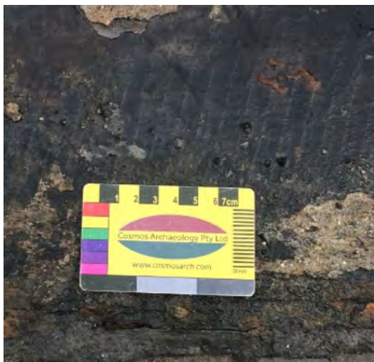
Figure 4.65: Pitsaw marks on plank [529] S-O-S2-A. (Source: AMBS).
