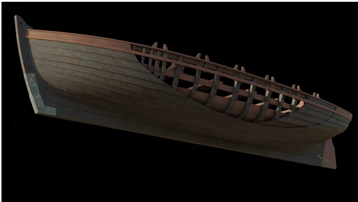
Figure 18: Port cutaway view of reconstructed vessel showing framing and double planking. Reconstruction and 3D rendering by B. Wharton and K. Edwards.
