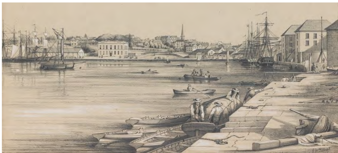
Figure 5.46: View in Sydney Cove, NSW, by Jacob William Jones 1845. Note the number of lighters operating and the two craft at base of image showing ceiling planking does not extend above the turn of the bilge.
