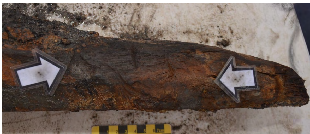
Figure 4.27: Tool marks on upper port side of stern knee [301]. Presumably from an adze or hand axe/hatchet. (Source: Casey & Lowe).
