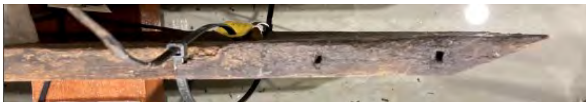
Figure 4.59: Starboard plank [338 S-I-S10-M] with 2 x \frac{1}{4} " square nail holes on top edge. (Source: Benjamin Wharton 2020).
