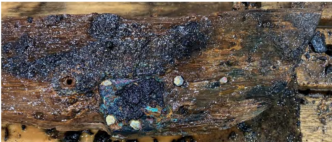
Figure 4.15: Plank [539] with copper sheathing and sheathing tacks intact. Rake and curvature of stem can be seen at the foremost end (right). (Source: Benjamin Wharton 2020).
