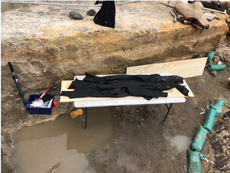
Figure 2.22: Timbers being wrapped in unwoven ‘felt-like’ geotextile. Although the material shed fibres, it was found to retain water better than hessian. The retention of water was seen as a priority as it was unknown how long the timbers would stay in cold storage. Potential for mould growth was also a concern and hessian is more susceptible to such a process than geotextile.
