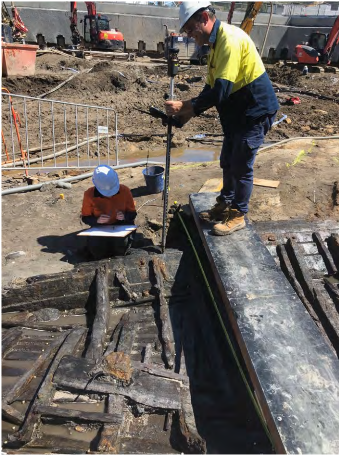
Figure 2.19: Taking the 'lines' of the hull – from the inside – using a Total Station. Note the brass tacks placed in the hull from where spot heights are to be taken.
