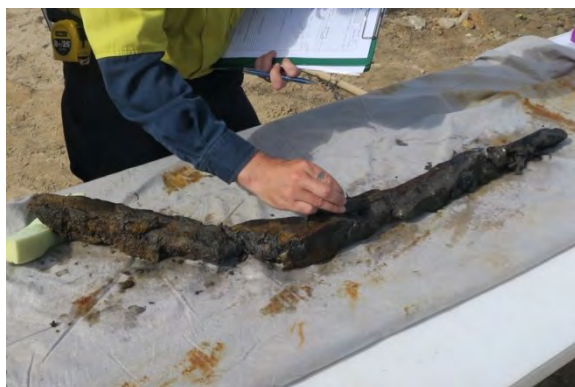
Figure 2.79: Assessing wood softness with pin.
