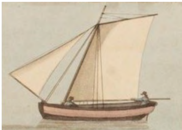
Figure 5.29: Detail from illustration of Sydney Cove viewed from the east. Gaff-rigged mainsail with headsail affixed to a bowsprit. Note the standing rigging required. No evidence has been found to date of standing rigging on UDHB1.
