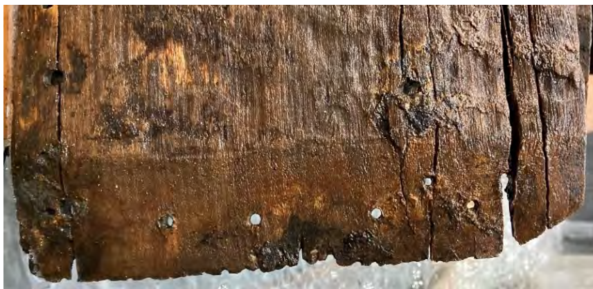
Figure 4.67: Scarf showing perpendicular grain having been quarter sawn [498 SI-S7-M]. (Source: Benjamin Wharton 2021).
