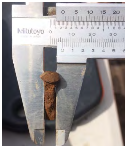
Figure 4.72: \frac{1}{4} " hand forged iron square shanked nail with rosehead. Catalogue #2245. (Source: AMBS).
