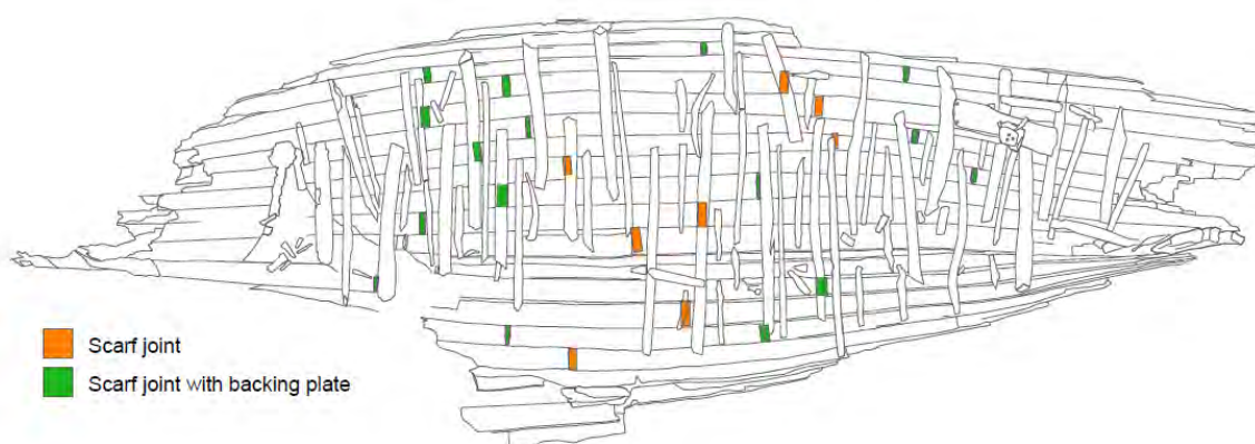
Figure 4.50: Scarf joint layout. Diagram shows placement of frames over scarf joints, and scarf joints with scarf plates. (Source: Benjamin Wharton 2020 using Casey & Lowe base plans: Plan_16.W5 and Plan_16.W6).
