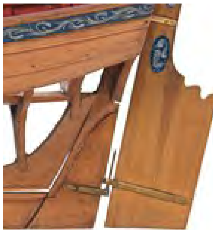
Figure 4.37: Gudgeon and pintle on model longboat.
