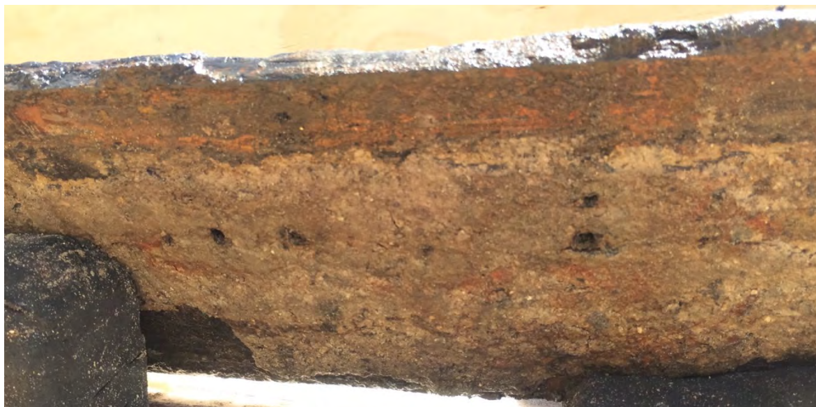
Figure 4.122: White putty between planking layers on outside of inner plank [311 P-I-S2-A]. Note also the fastener holes protruding through from the outer layer planking. (Source: AMBS).
