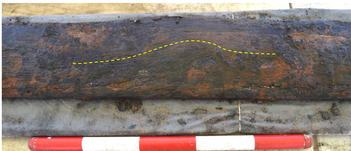
Figure 4.69: Garboard plank [407 P-I-S1-M] of the port side. Swirl evident on plank (direction shown with yellow dashed line) around a 'sound' knot in Sydney Blue Gum. (Source: Casey & Lowe).
