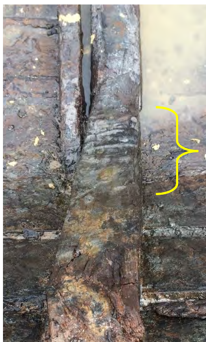
Figure 4.94: Branch collars on futtock frame [399] FT-A. (Source: AMBS)
