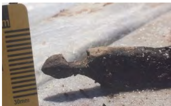
Figure 4.44: \frac{3}{8} " treenail hole in stem knee [456]. Scale in 1 mm increments. (Source: AMBS).
