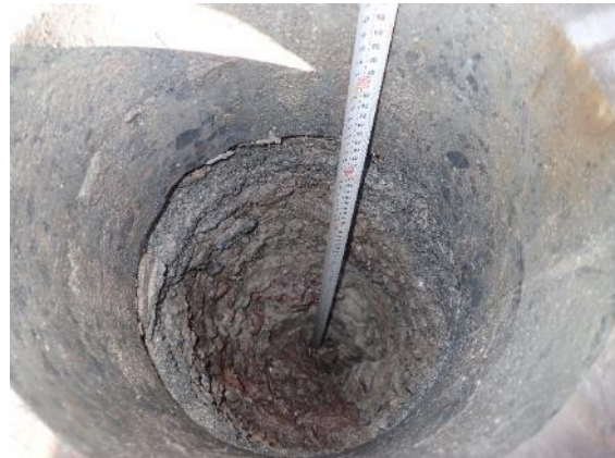
Figure 5.5 Introduced clays present in excavated borehole.
