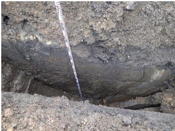
Figure 5.8 Dense grey clay in TP13, below a crumbly grey fill that included some industrial materials.
