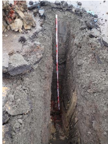
Figure 5.7 Mix of introduced C Horizon greys, red and yellow clays in TP10.
