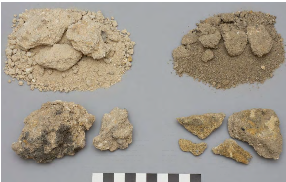
Figure 3.8: Selected mortar examples (l-r). Top row: powdery shell sand 097/#1030, firm shell sand 009/#1005. Bottom row: firm lime sand 009/#1004, 020/#1008. 100mm scale. DSC_4122. Russell Workman.
