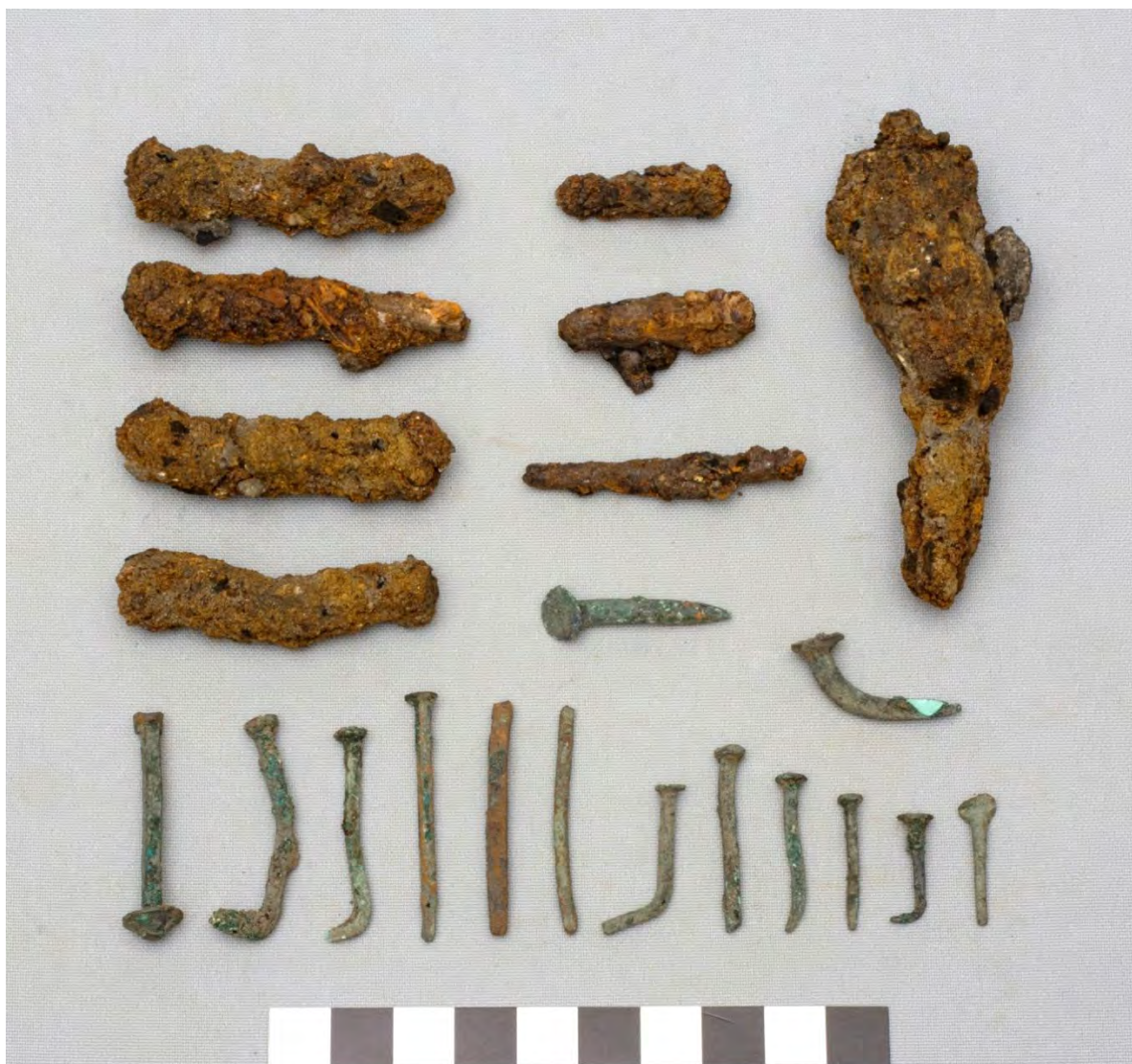
Figure 4.2: Metal nails and tacks from accumulated sand deposit (337) showing the difference in preservation between iron and copper alloy from the same archaeological deposit. (l-r) Top left: four nails #10737. Top centre: three iron nails #10739. Top right: iron nail #10738. Middle: two WD sq countersunk sheathing tacks #10736. Bottom row: WD sq nails - nail and conical rove #10725, #10726, #10727, #10728, #10729, #10730, #10731, #10732, #10733, #10734, #10735 (two). Scale 100mm. DSCN_3088. Russell Workman.
