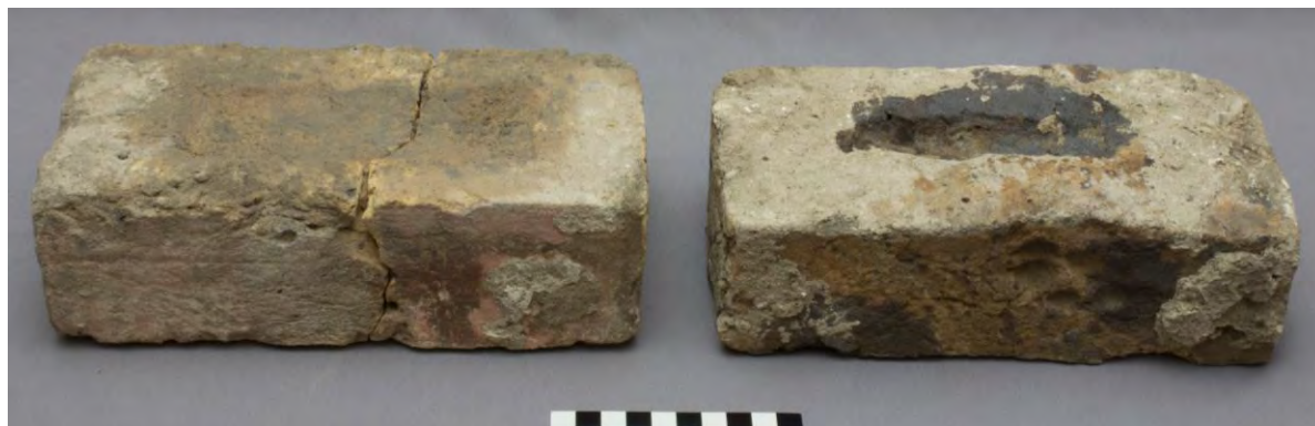
Figure 3.2: The rectangular frogged sandstock bricks that formed the floorboard support pad for House 1 Room 2 072/#1028, 072/#1029. 100mm scale. DSC_4077. Russell Workman.
