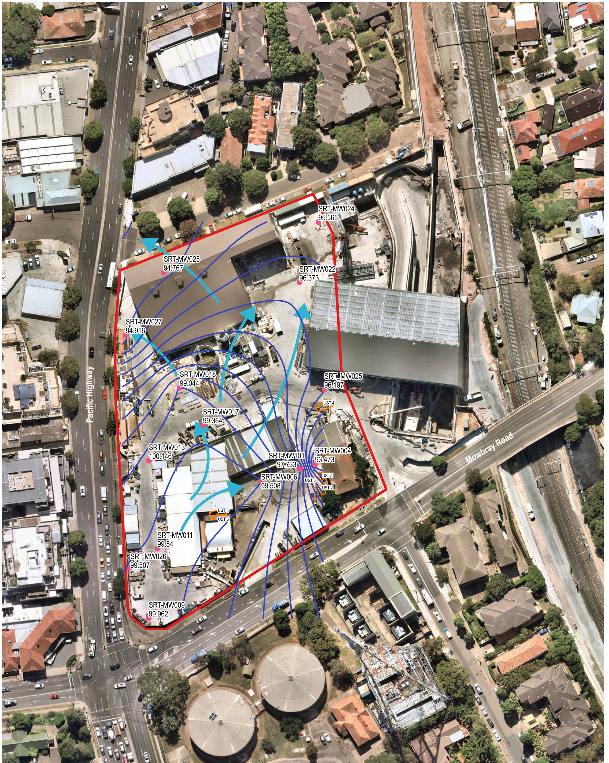
Figure 3b: Stage 2 Inferred Groundwater Levels
