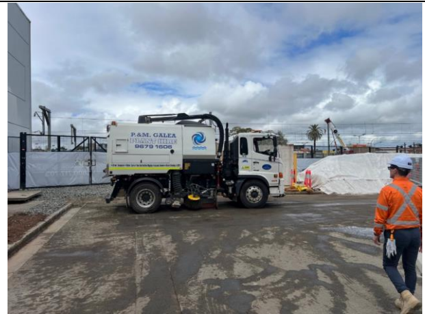
The street sweeper was in use during the inspection to remove mud spilt onto the main access
