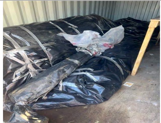
Storage of Quenos pipe contaminated with asbestos and coal tar (awaiting disposal in QLD)
