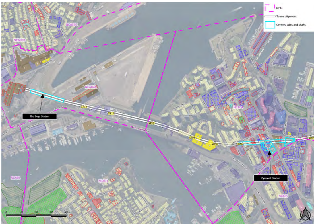
Figure 2.1: Mainline tunnel alignment, cross passages and caverns - The Bays to Pyrmont Station
