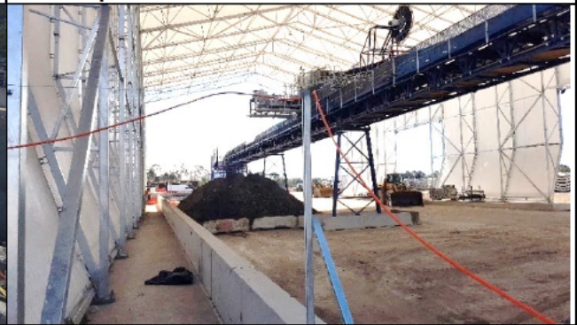
View north inside Orchard Hills tunnel spoil shed and conveyor system with spoil storage underway
