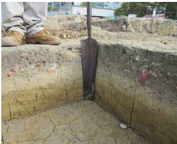
Figure 2.3 Example of the PSB Pleistocene or Tertiary Alluvium excavated at Parramatta Square. (Source: Lawrie 2019 6 )
