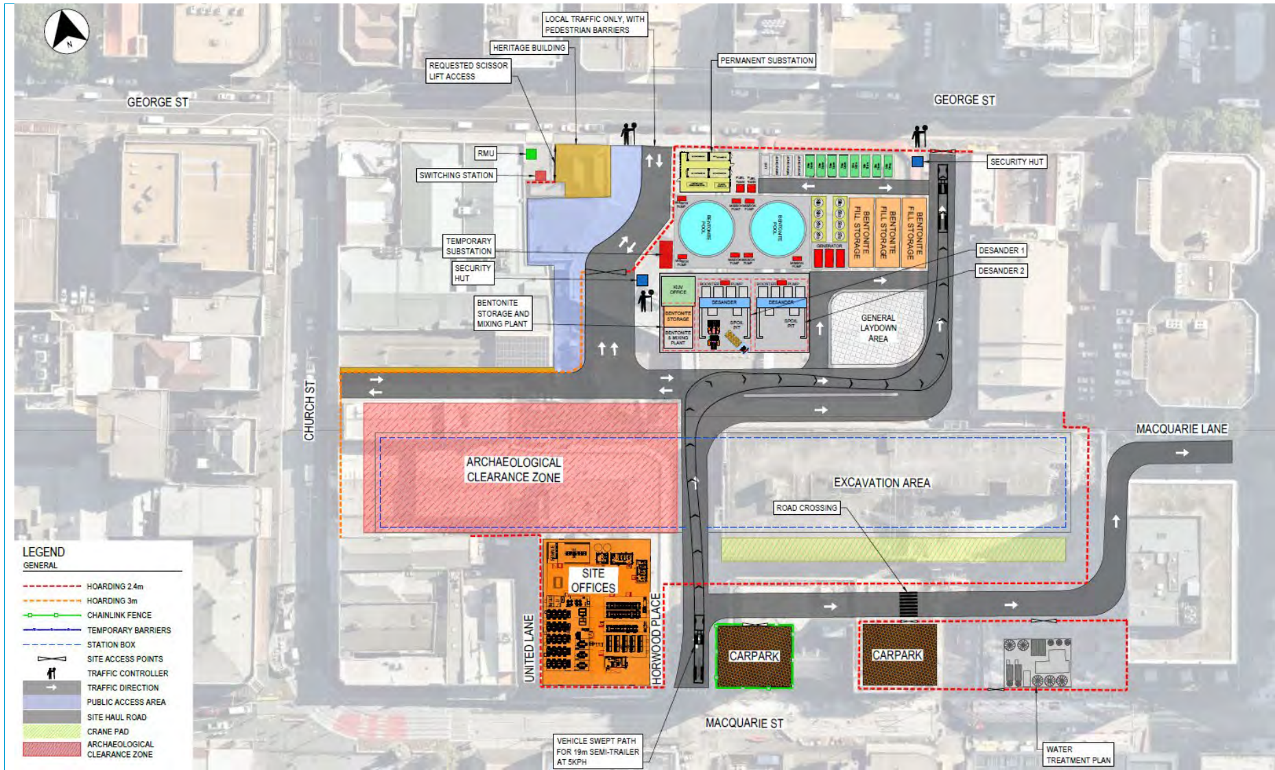
Figure 2: Parramatta indicative construction site.
