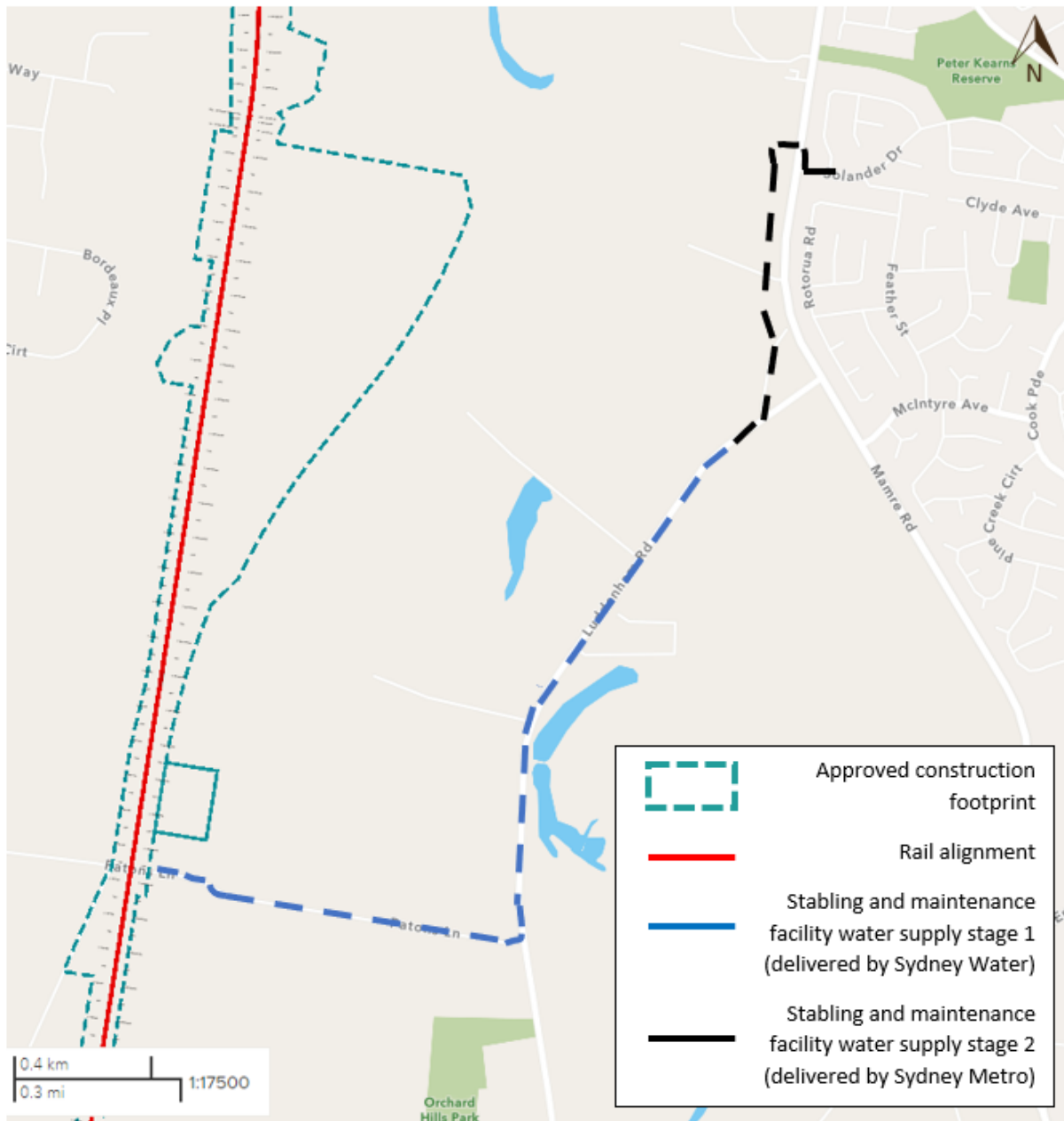
Figure 2 Assessment and delivery strategy for the proposed stabling and maintenance facility water supply.
