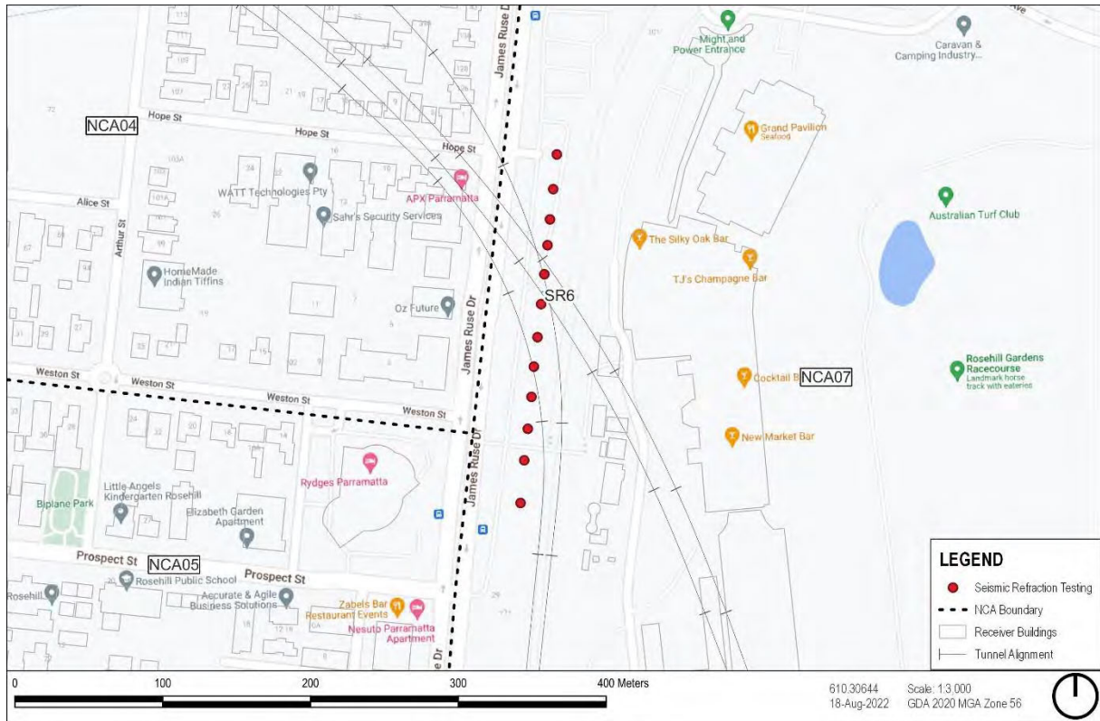
Figure A5 Seismic Refraction Testing (SR6)
