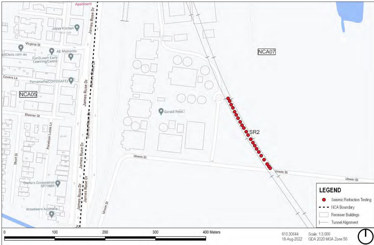
Figure A2 Seismic Refraction Testing (SR2)
