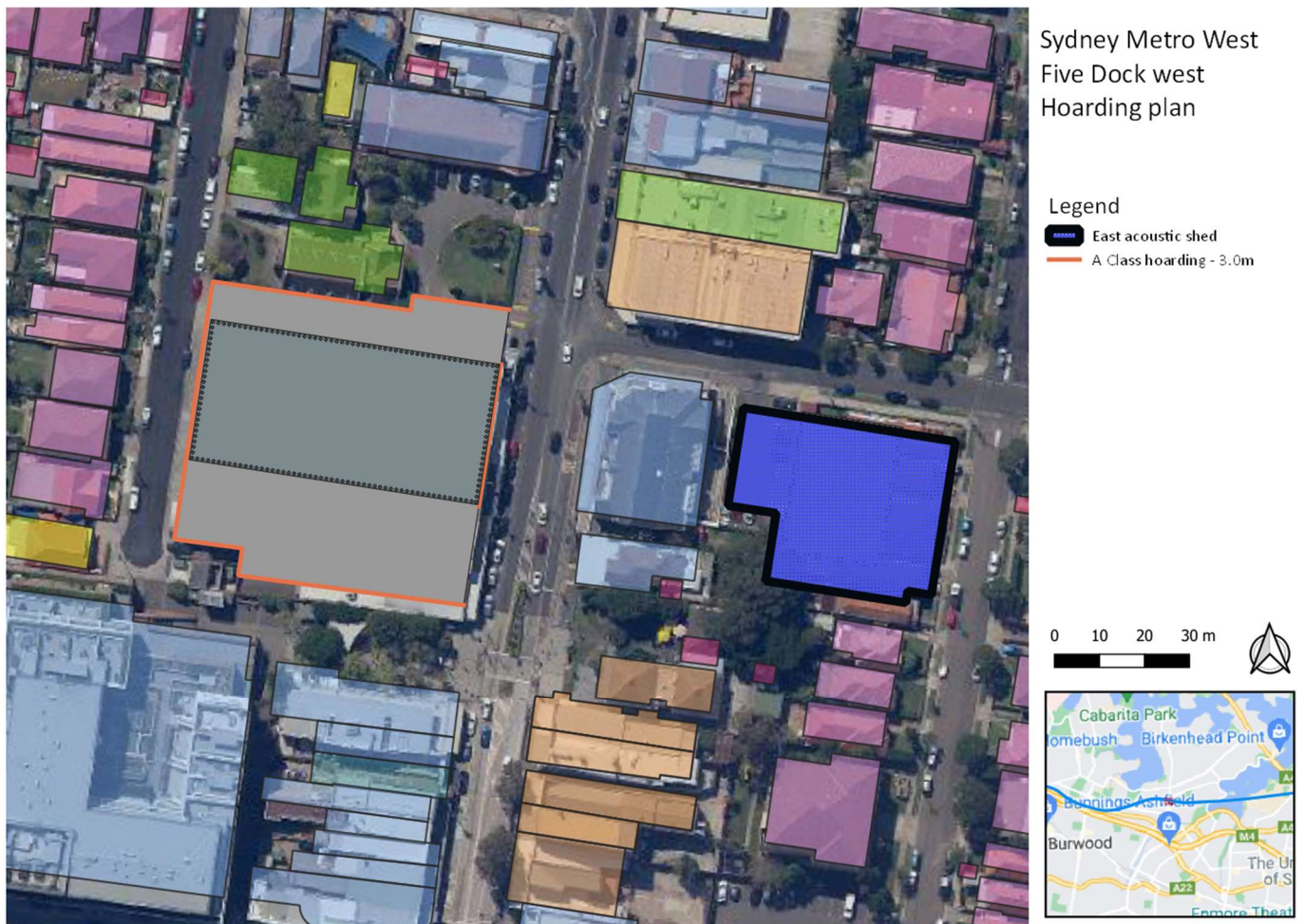
Figure 5-1 Hoarding arrangement Five Dock west and acoustic shed east
