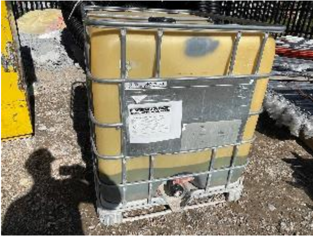
Plate 27 – Unbunded chemical container
