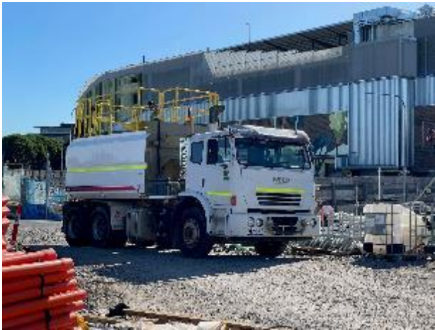
Plate 36 – Water cart in use for dust suppression on hardstand area near old WTP
