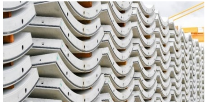
Tunnel segments at the precast facility in Brisbane.
