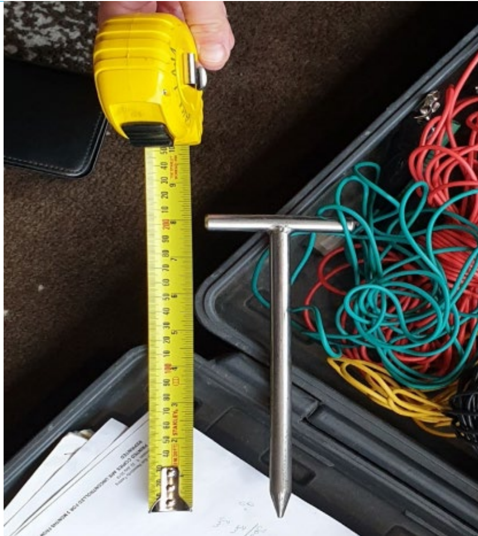
Figure 3: Example of an electrode used for soil resistivity testing
