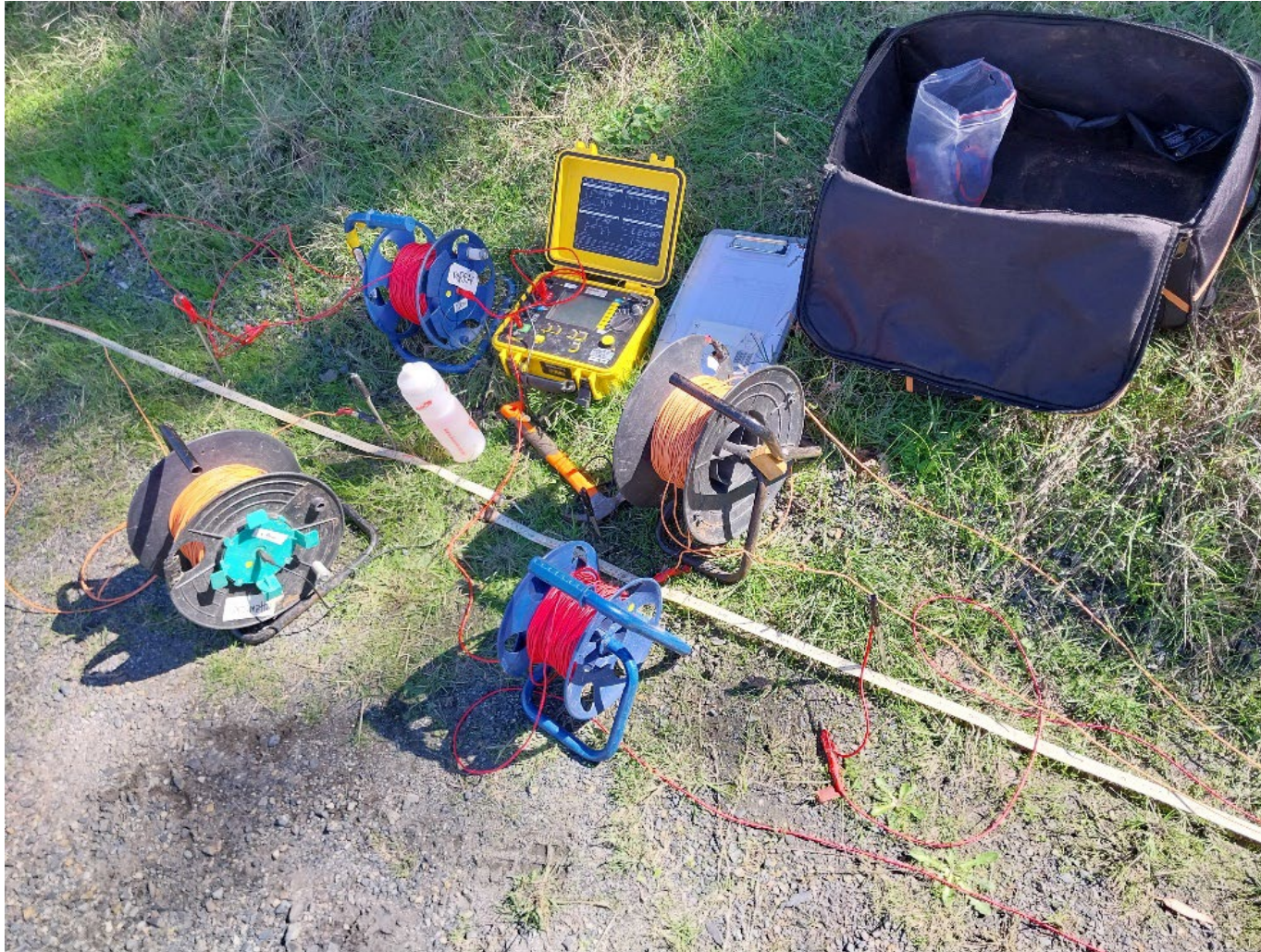
Figure 4: Example of a soil resistivity testing set up
