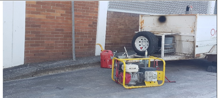
Clarke Lane South – Unbundled storage of Flammable liquids
