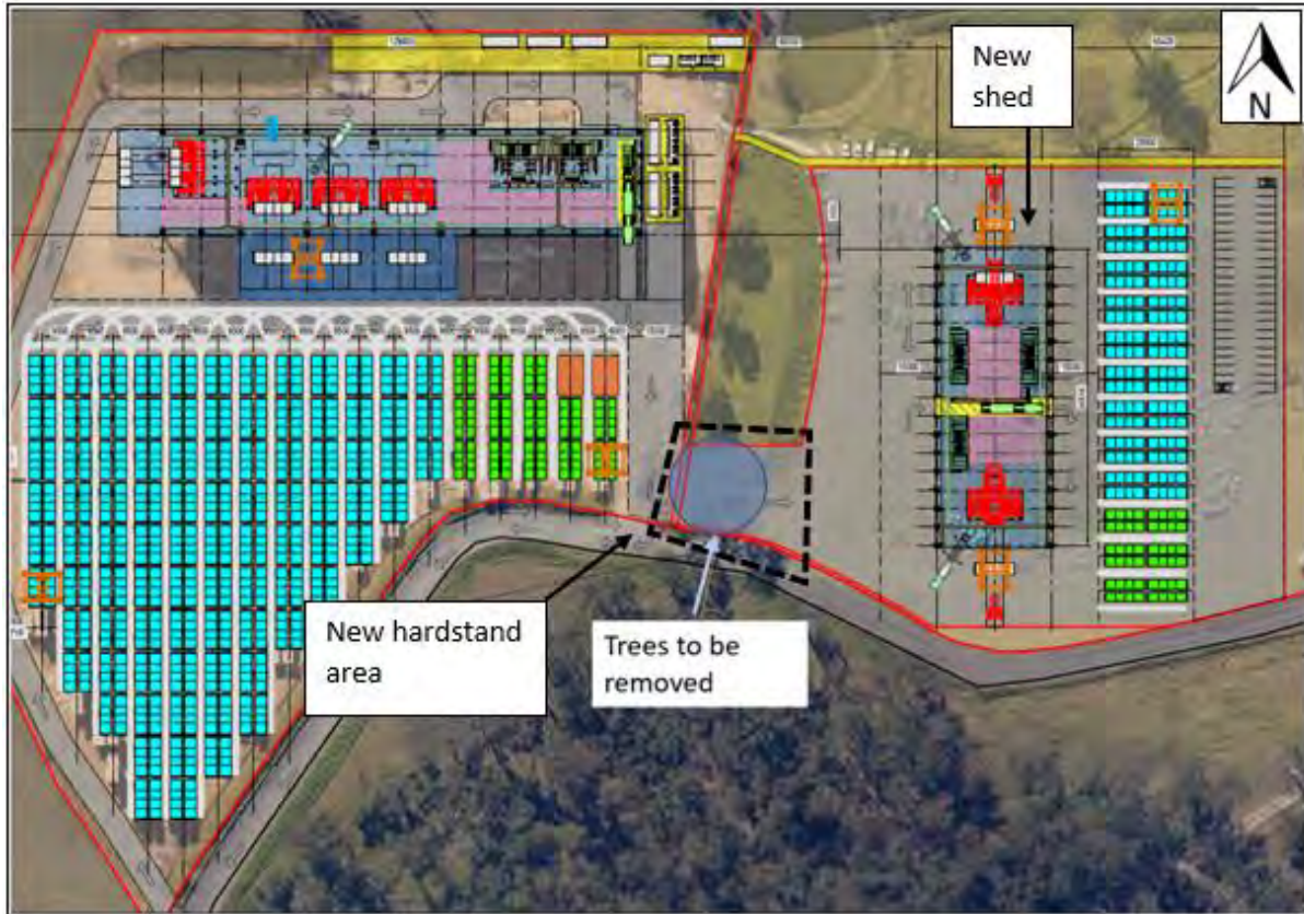
Figure 2: Location of proposed change, showing location of the new temporary shed, new hardstand area, and location of vegetation removal
