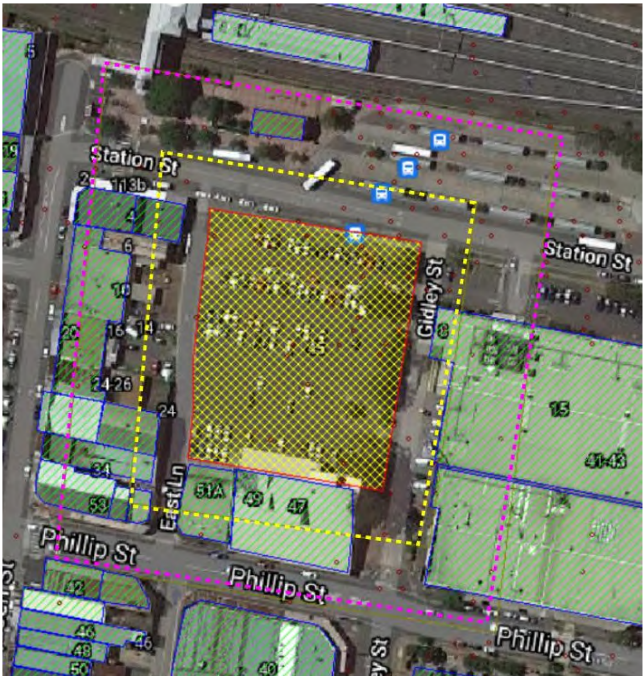
Figure 9-1 Vibratory Roller Building Damage Risk – Yellow Line Indicates 15 m Buffer for Commercial Buildings; Pink Line Indicates 41 m Buffer for Heritage Items
