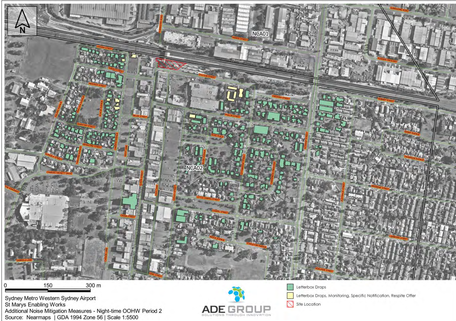
Figure 31 Additional Noise Mitigation Measures, Night-time Out of Hours period extent (Residential receivers)
