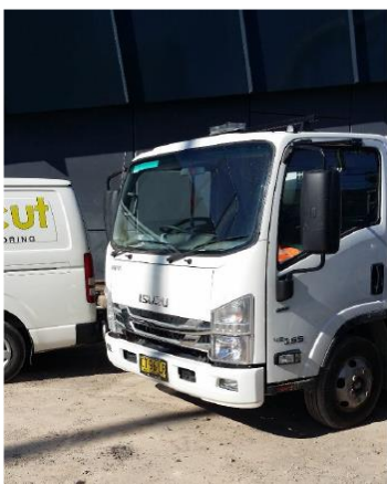
LHS: Truck - one of two (2) vehicles observed not to be fitted with quackers (high tonal reverse beepers were audible on the day).
