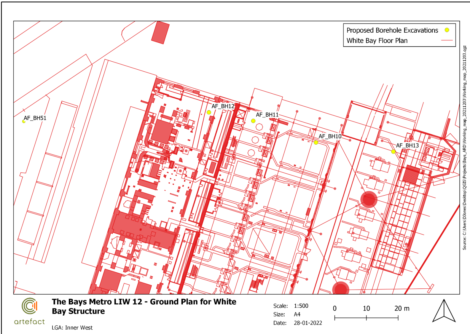
Figure 4: Plan of the White Bay Power Station Power House ground level with borehole locations.
