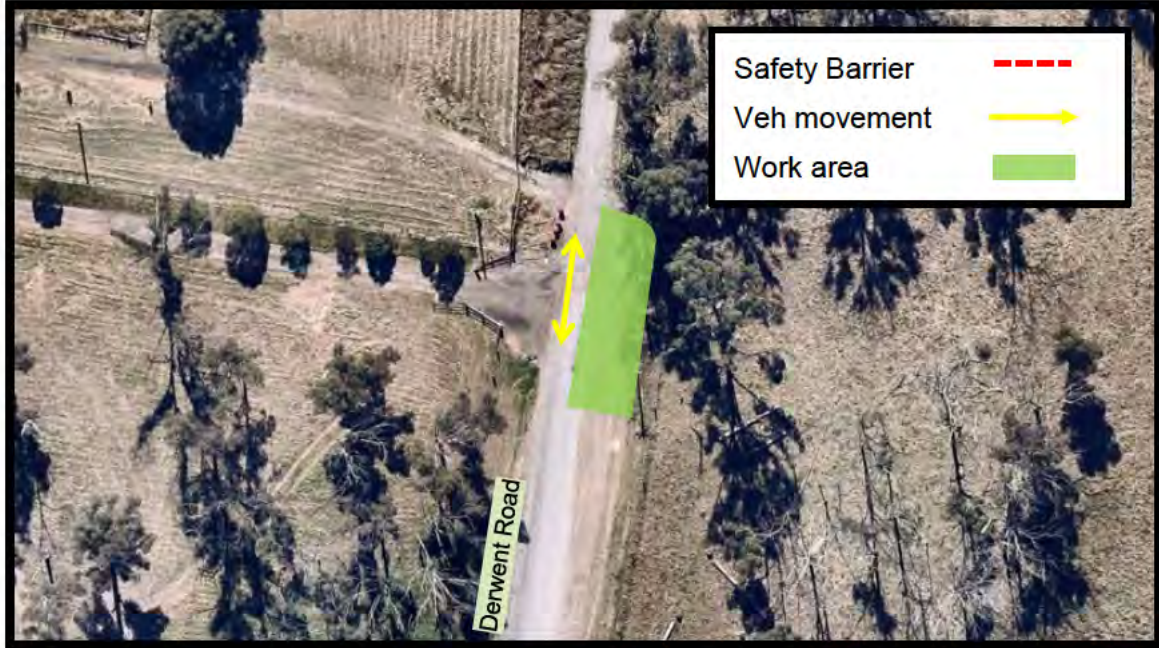
Figure 13 – Derwent Road access construction - Stage 1
