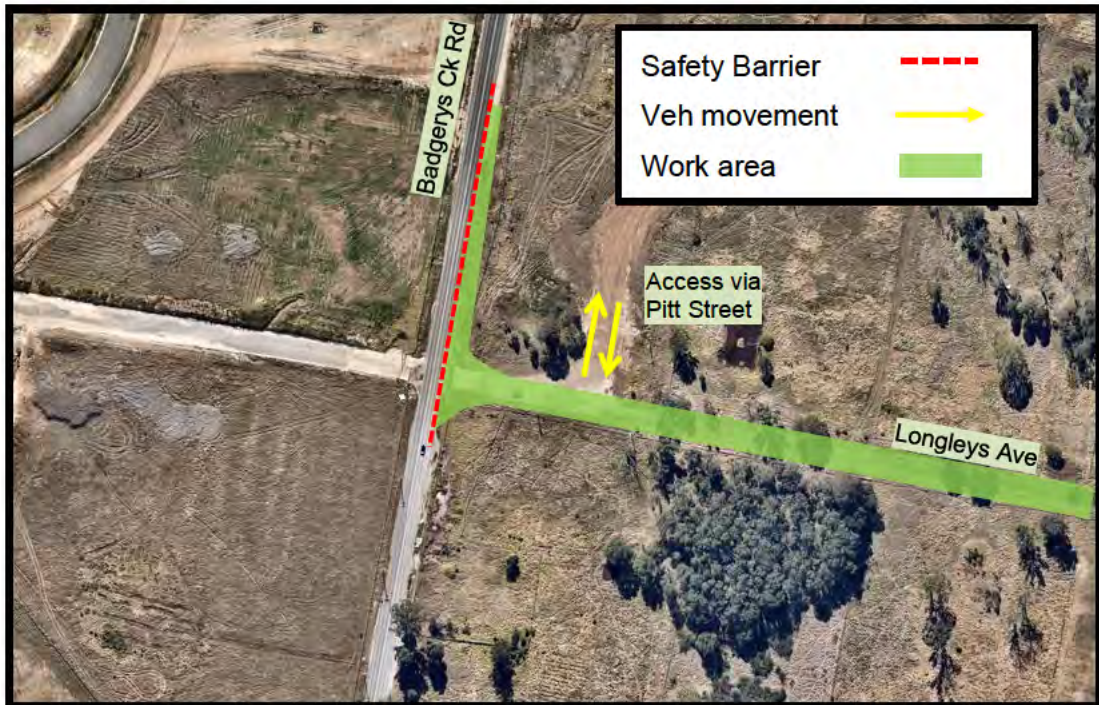
Figure 8 – Badgerys Creek Rd / Longleys Ave Stage 1 Construction
