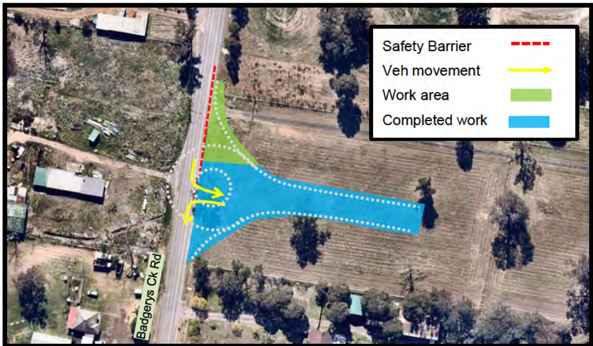
Figure 11 – Badgerys Creek Rd / Aerotropolis Roundabout Stage 2 Construction
