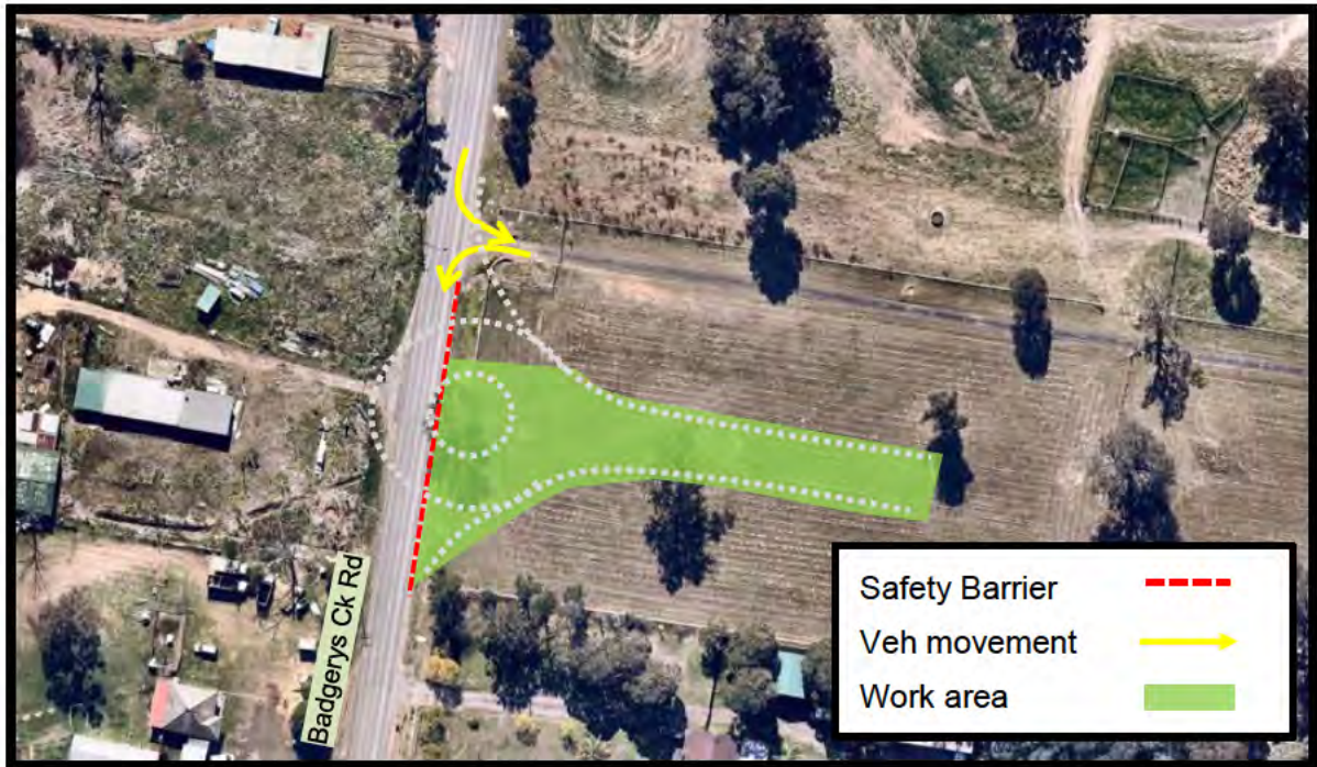
Figure 10 – Badgerys Creek Rd / Aerotropolis Roundabout Stage 1 Construction
