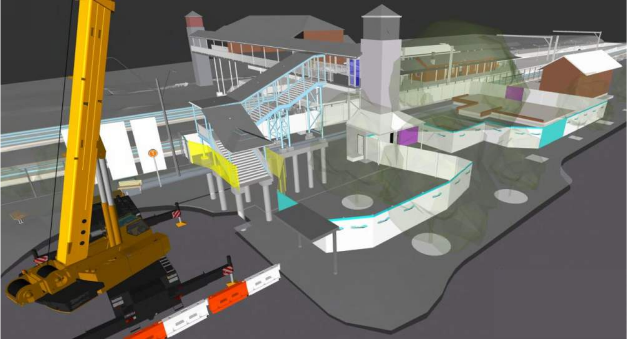
Figure 10 - Pedestrian switch to new staircase
