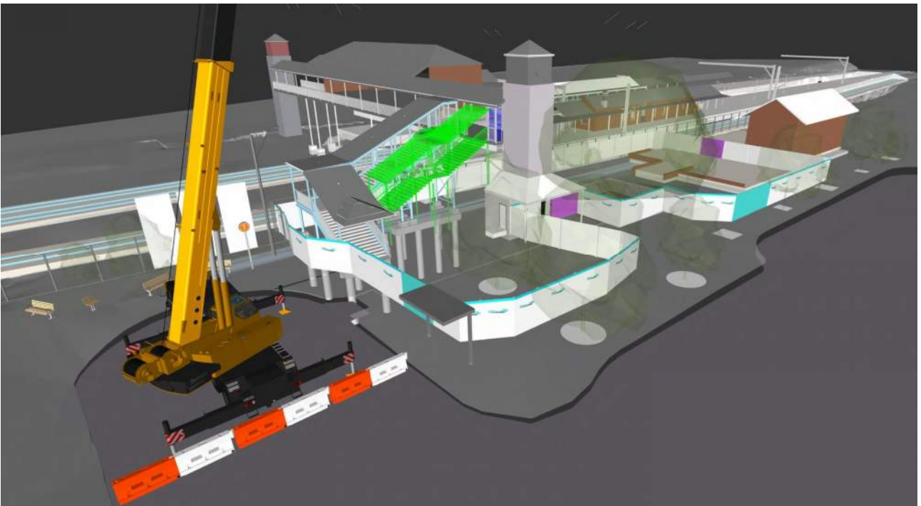
Figure 11 - Demolition of existing stairs
