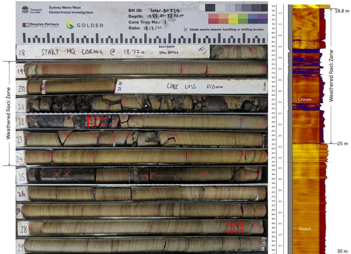
Figure 8: Core and Acoustic Televiewer Log from SWM_BH724
