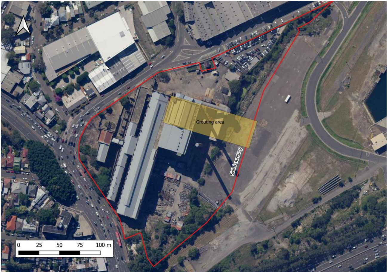
Figure 3: State Heritage Register boundary shown in red. Area proposed for grouting shown in yellow (plan prepared by Comber consultants).
