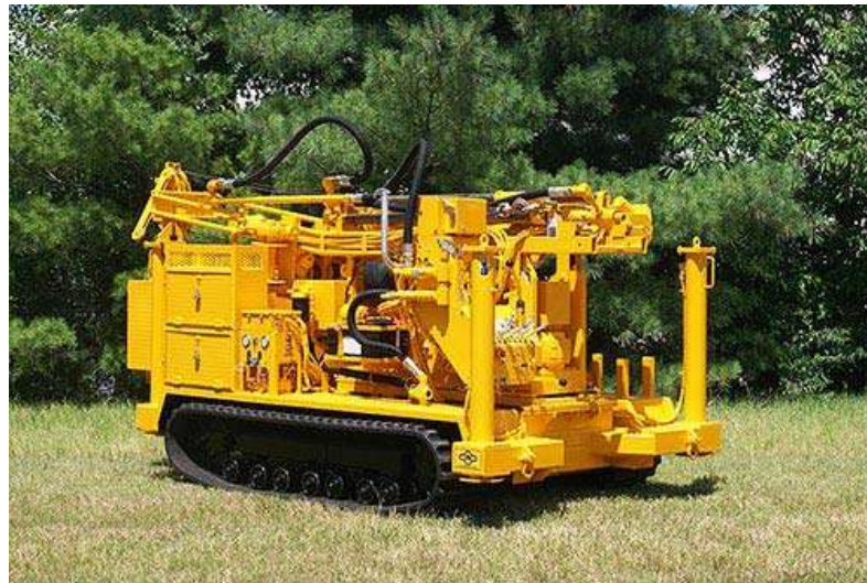
Figure 13: CME 45 Rubber-Tracked Drilling Rig
