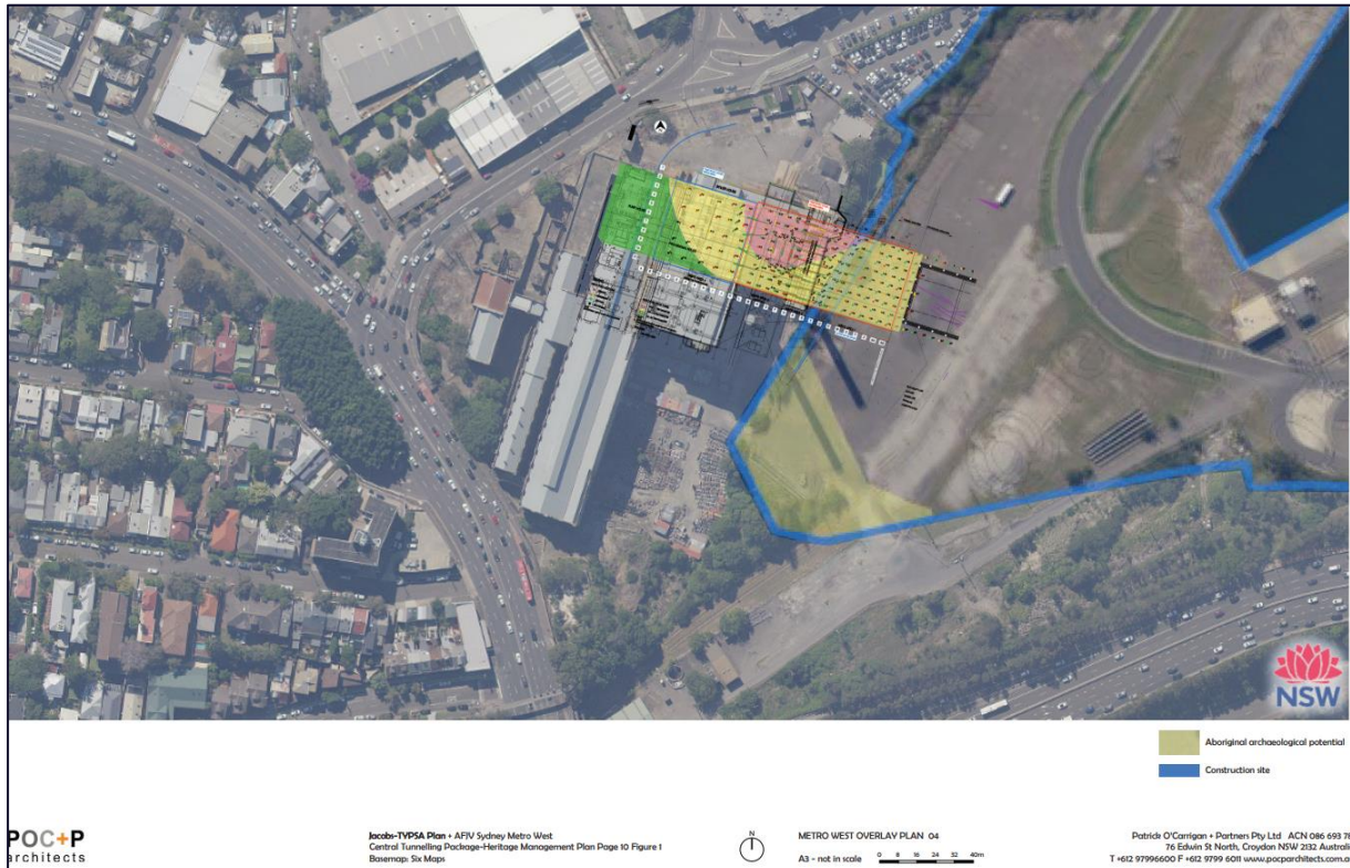
Figure 3: Showing location of proposed grouting and area of Aboriginal archaeological potential to the south of the grouting area (overlay by Patrick O’Carrihan + Partners)
