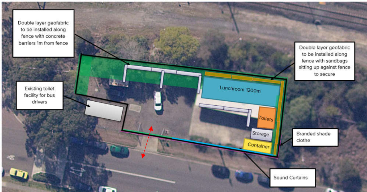
Figure 9: Station Street Laydown Arrangement
