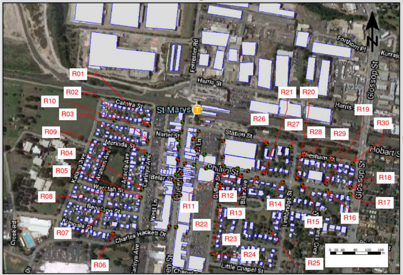
Figure 3 Representative Residential Receivers Surrounding the Works
