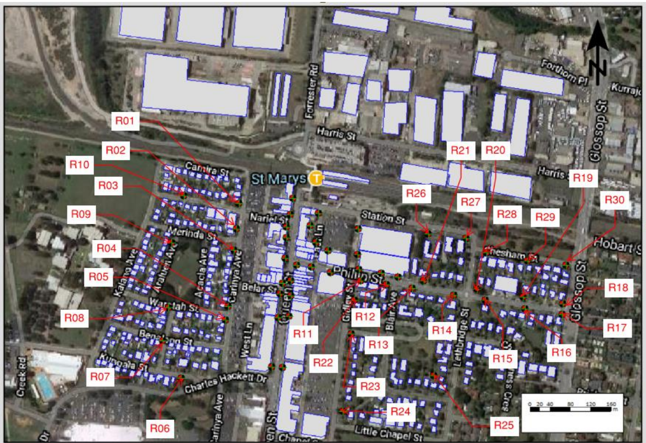
Figure 3-1 Representative Residential Receivers Surrounding the Works
