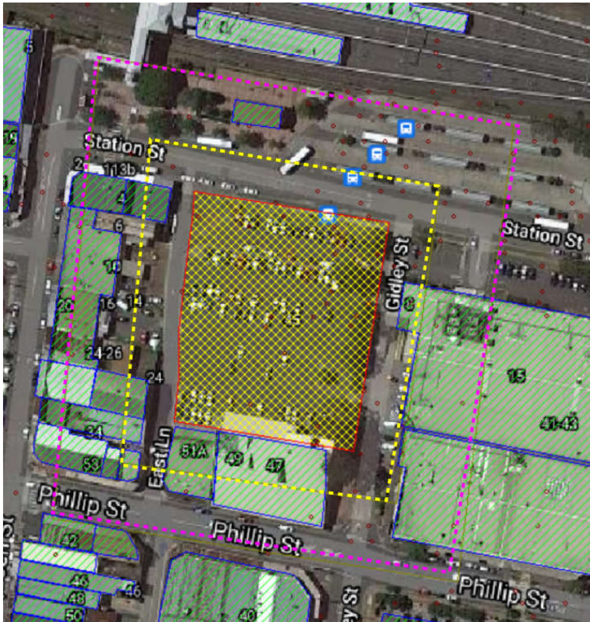
Figure 7 Vibratory Roller Building Damage Risk – Yellow Line Indicates 15 m Buffer for Commercial Buildings; Pink Line Indicates 41 m Buffer for Heritage Items
