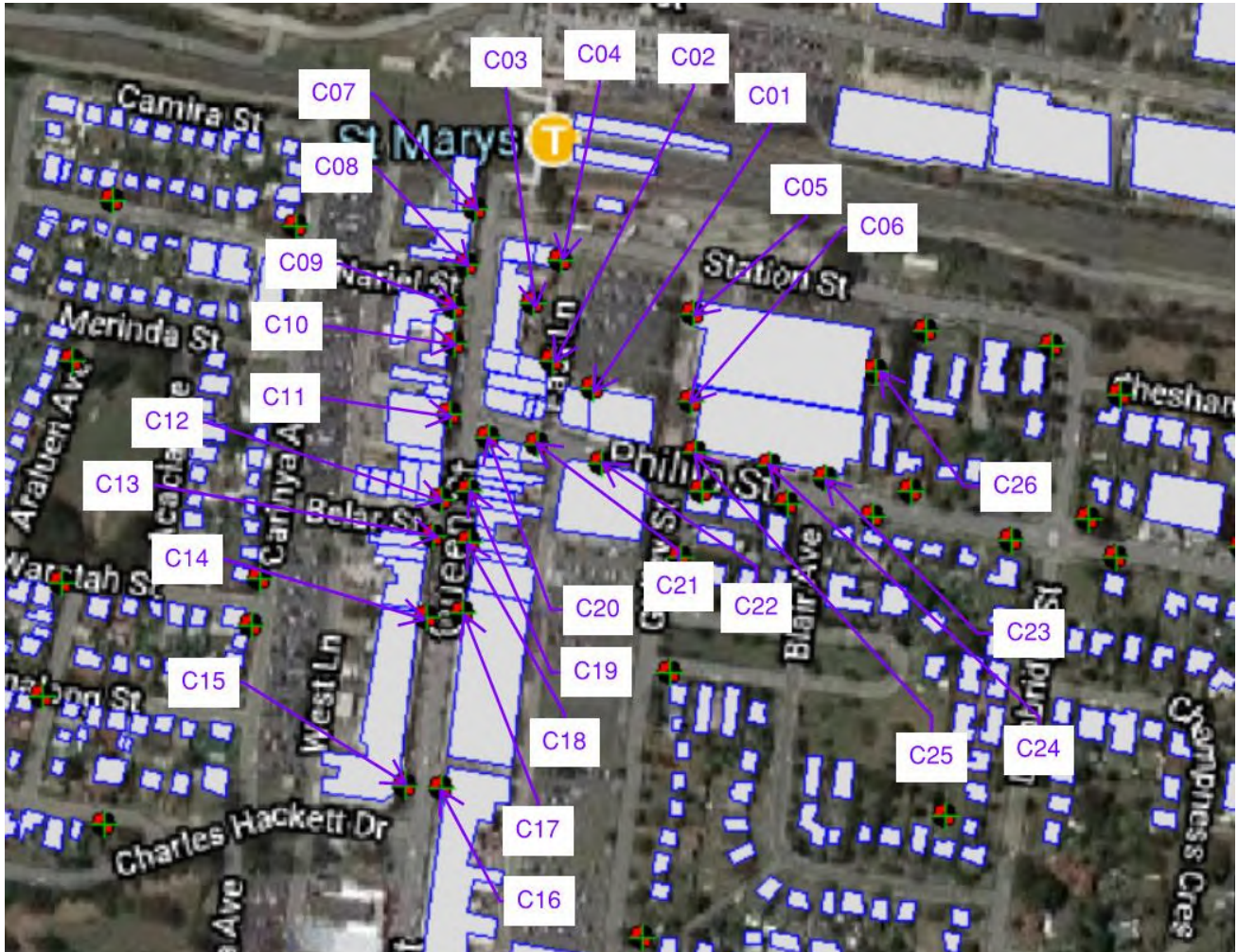
Figure 6-2 Representative Non-Residential Receivers Surrounding the Works
