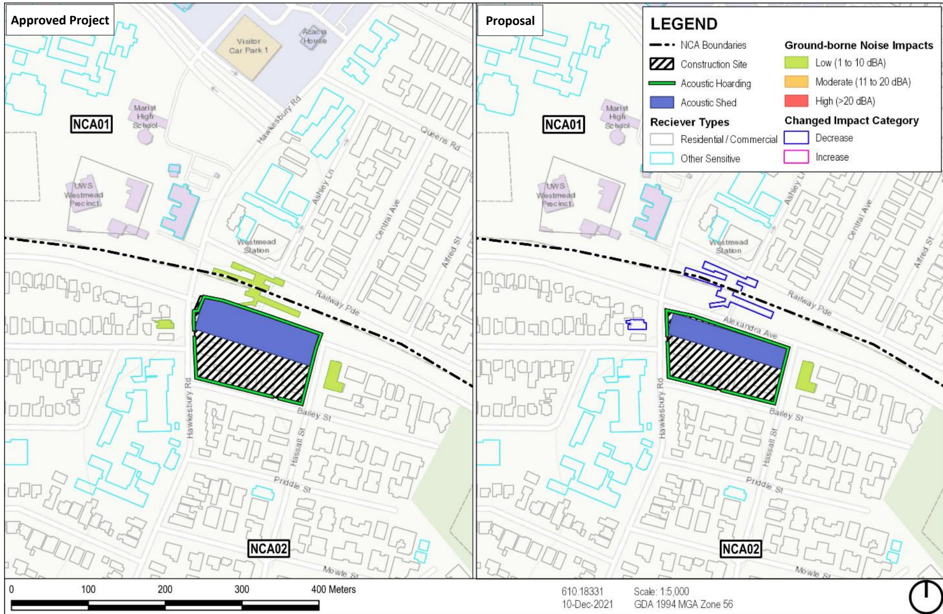
Figure 9 Ground-borne Noise Impacts – Daytime
