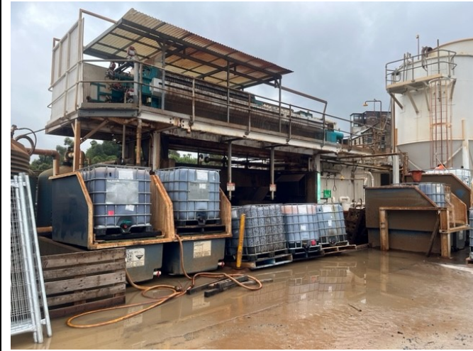
Chemical IBCs were observed without adequate secondary containment prior to the Christmas Shutdown
