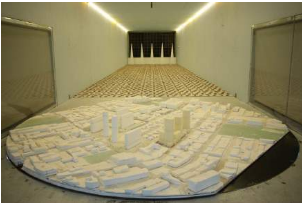
Figure 102 – Photograph of wind tunnel model (including the proposed OSD), from the north-west
