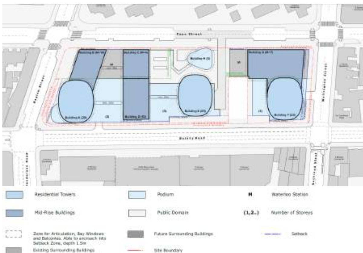
Figure 49 – Plan view of proposed building envelopes
