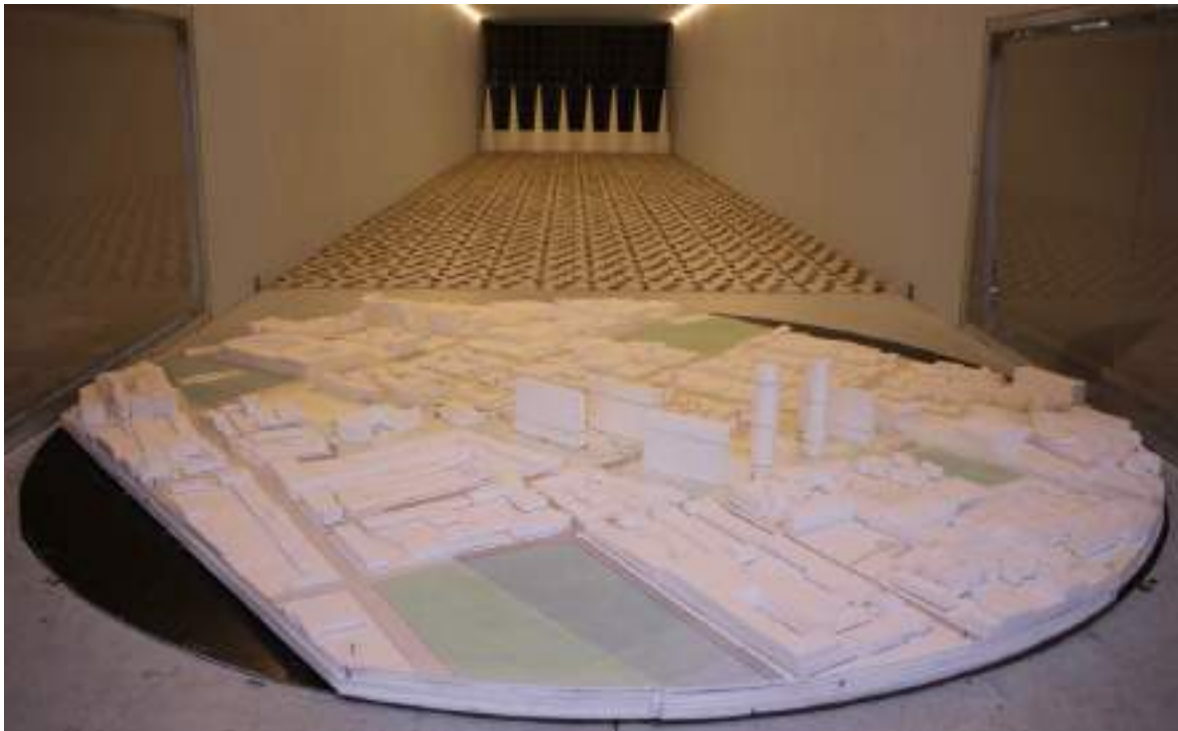
Figure 101 – Photograph of wind tunnel model (existing conditions), from the north-east
