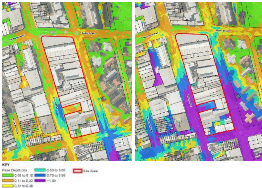
Figure 37 – Existing flood depths for 100yr average rainfall intensity (ARI) (left) and probable maximum flood (PMF) (right)
