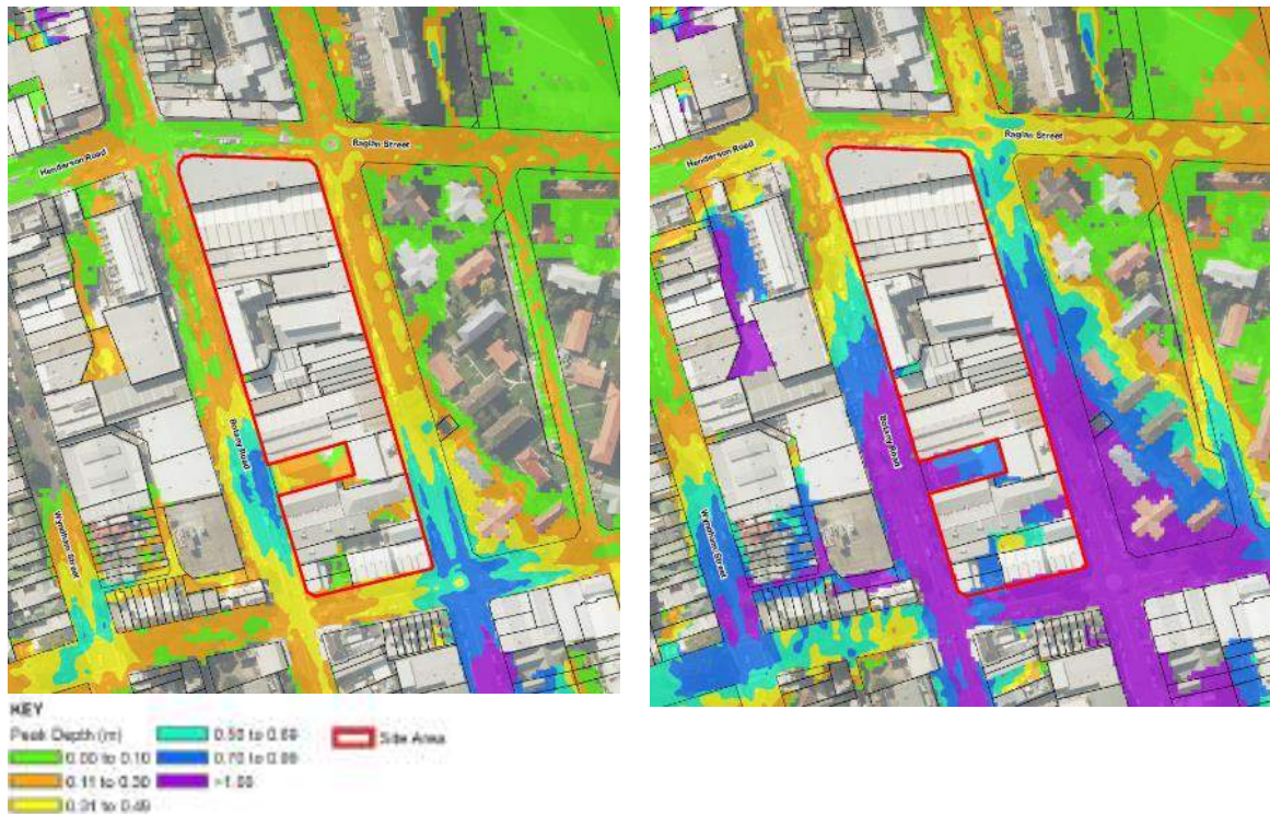
Figure 106 – Existing flood depths for 100yr average rainfall intensity (ARI) (left) and probable maximum flood (PMF) (right)
