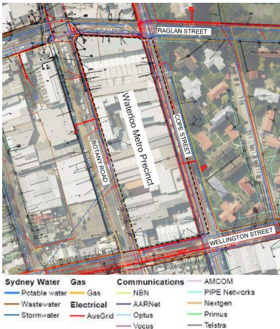
Figure 39 – Existing combined utilities and servicing plan
