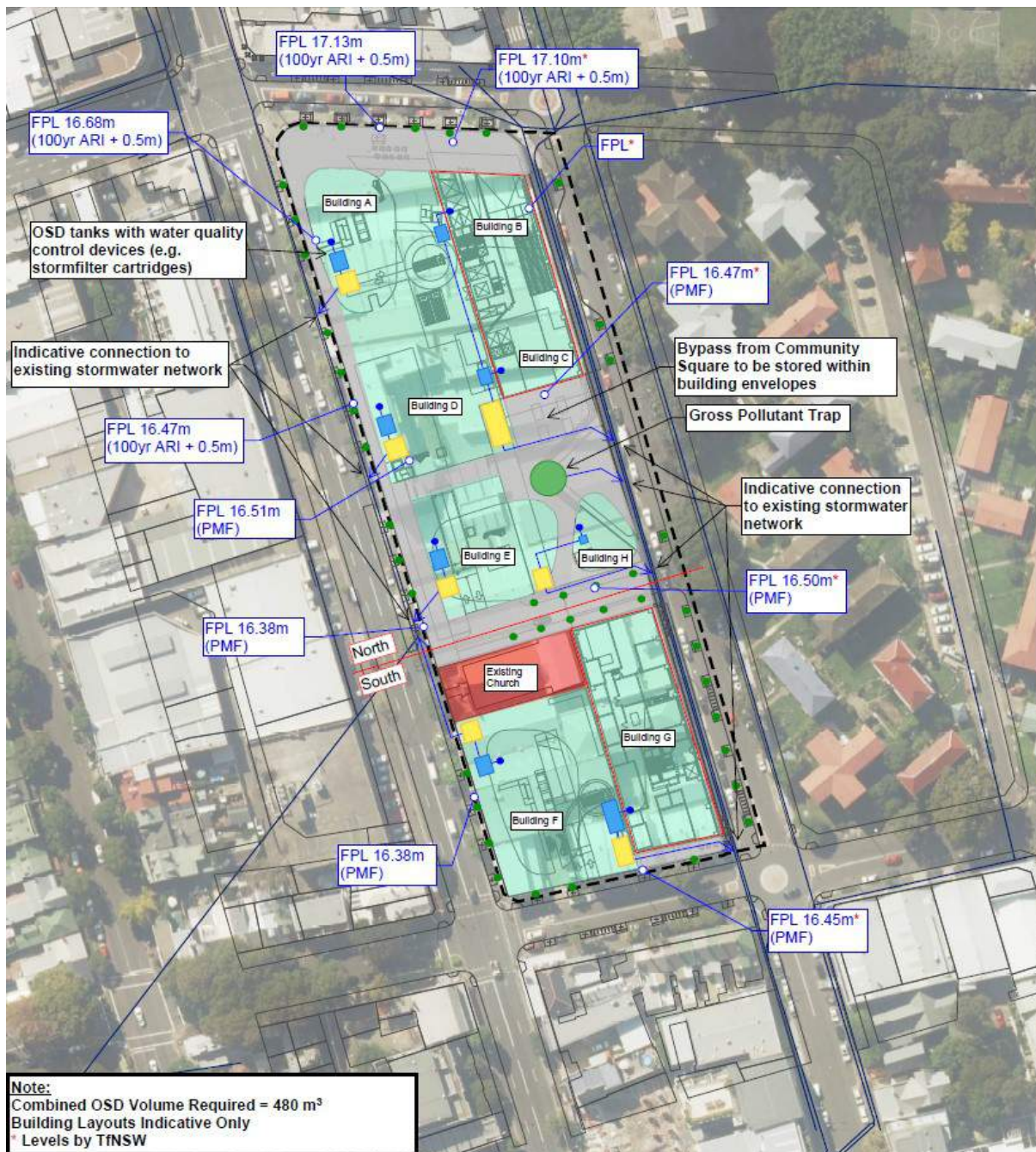
Figure 109 – Concept stormwater and flood management plan
