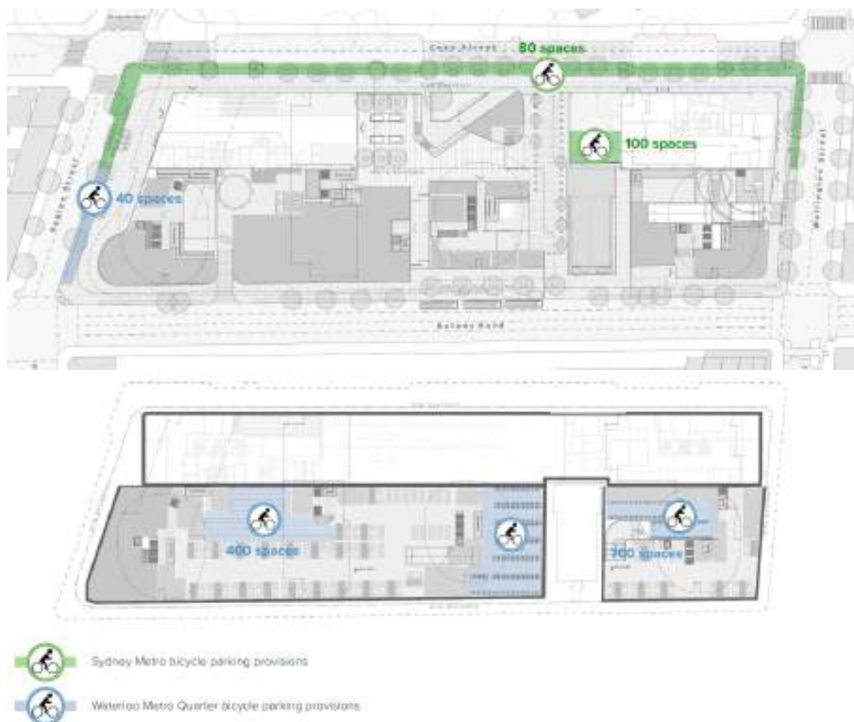
Figure 58 – Proposed locations of Metro Quarter OSD bicycle parking provision and Sydney Metro bicycle parking provision
