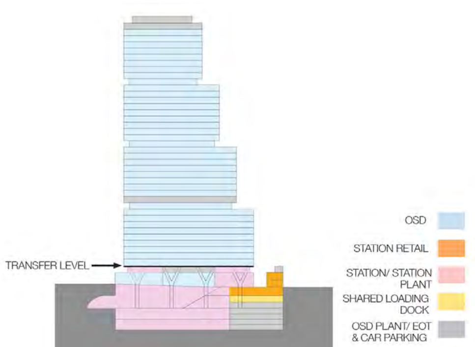
Figure 2: Delineation between the Metro station and OSD
