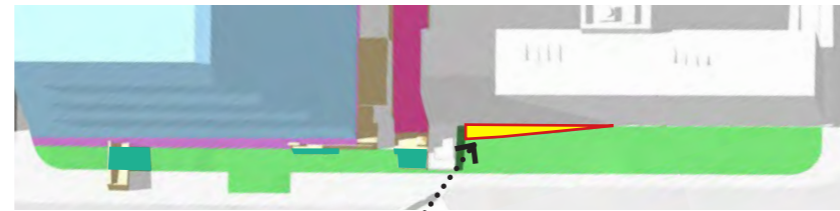
12.00pm March 21st Area of solar gain: 68.6 m2 Area of overshadowing : 33 m2
