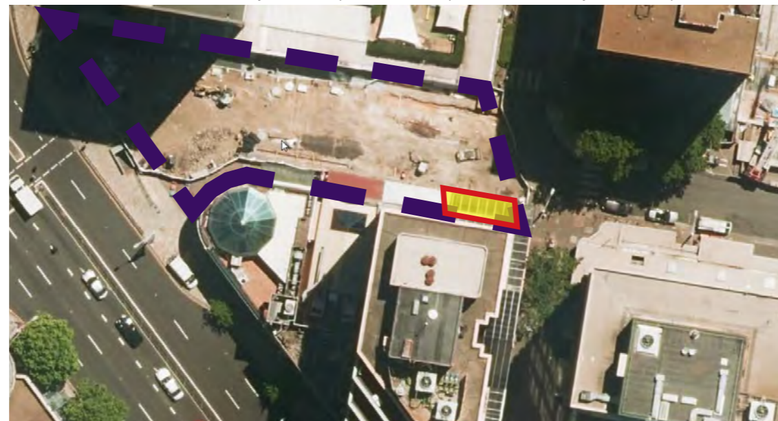
Overlay of extent of shadow created by the OSD concept SSSA building envelope on Brett Whiteley Plaza at 12pm June 21st
