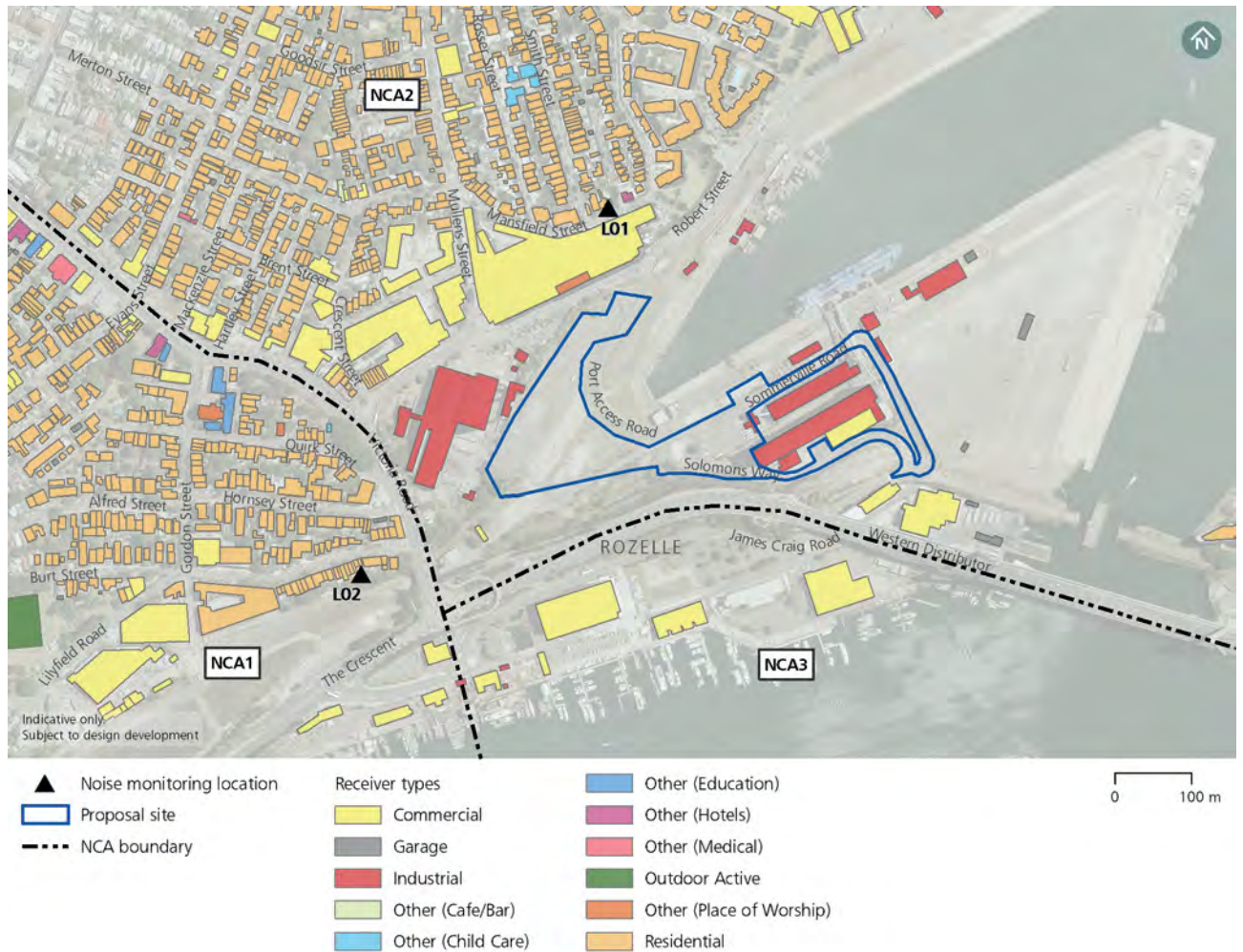
Figure 7-1: Noise Catchment Areas, receiver types and noise logger locations around the proposal
