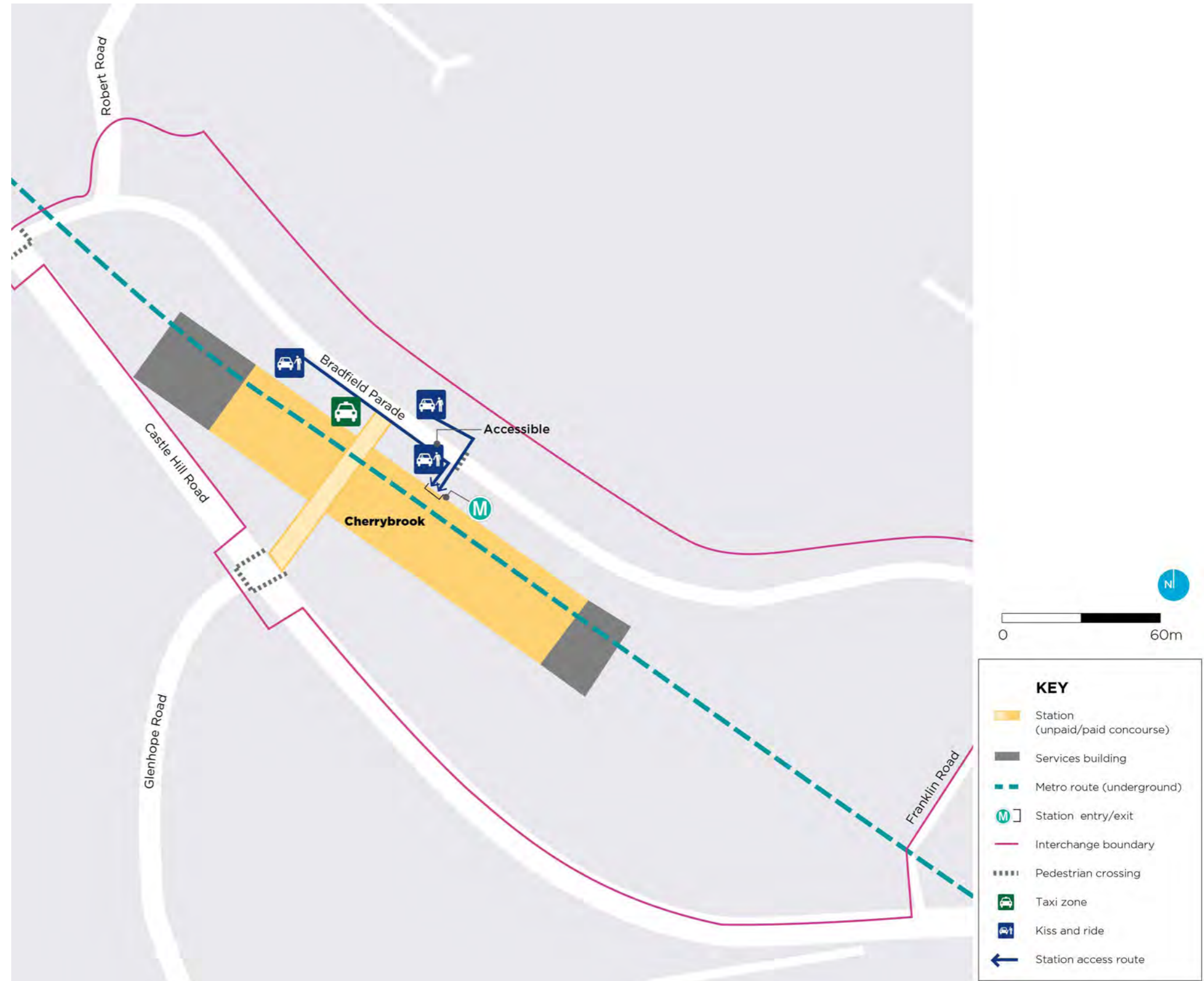
Cherrybrook Station - vehicle drop-off interchange and transfer requirements
