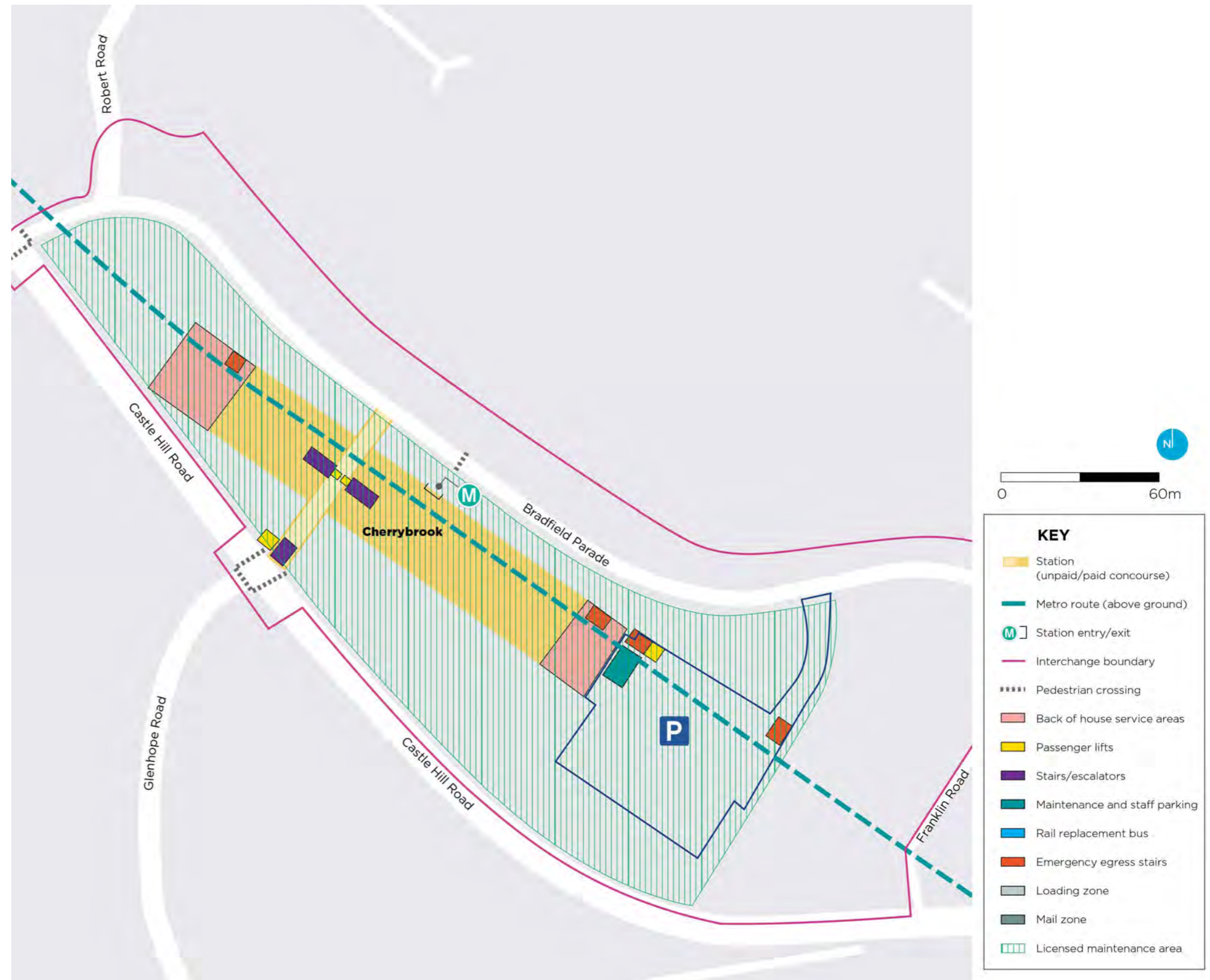
Cherrybrook Station - operations, maintenance and management provisions
