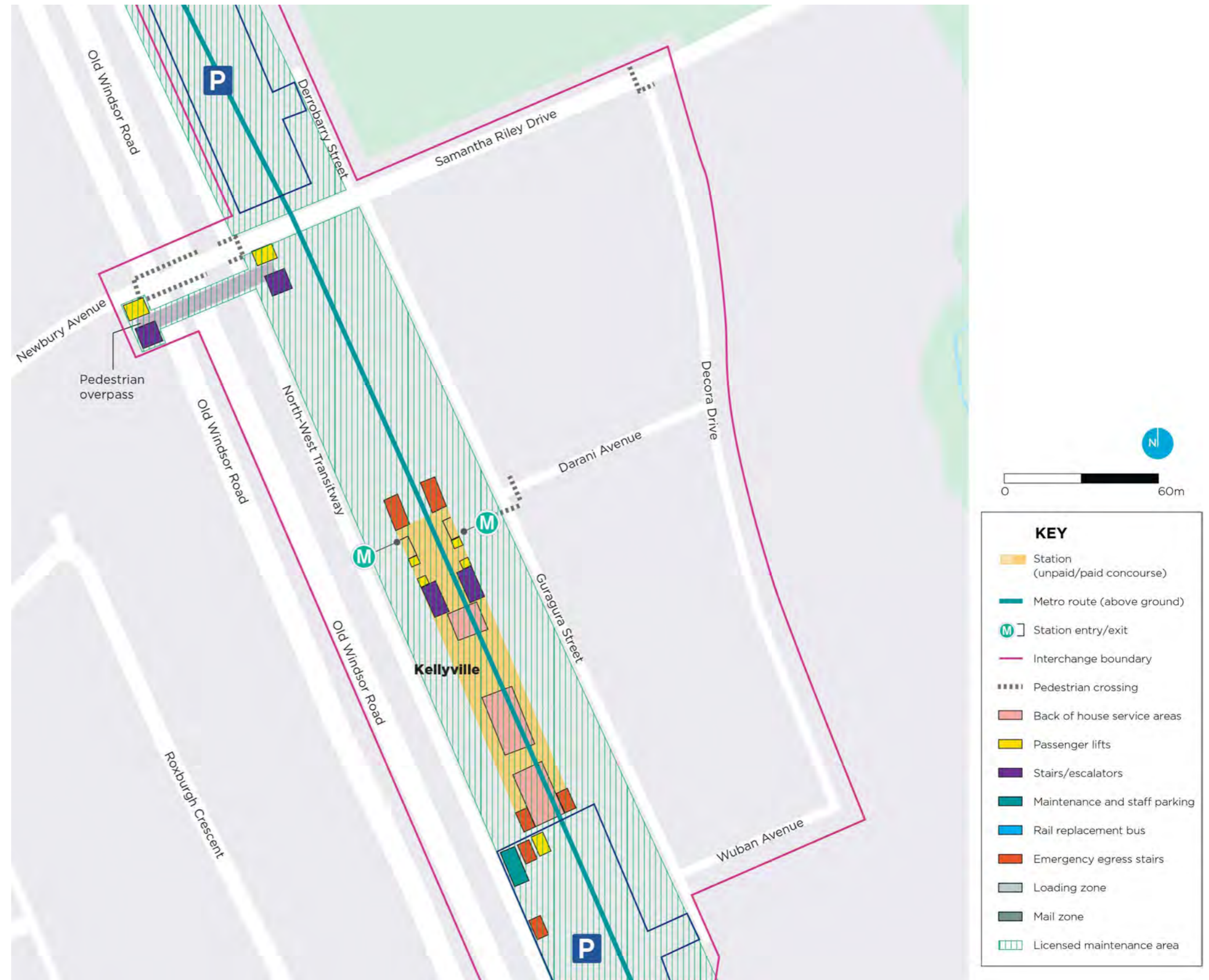
Kellyville Station – operations, maintenance and management provisions
