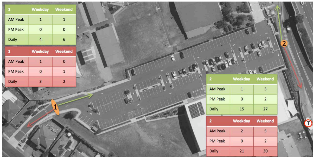
Figure 7-9 Bicycle volumes through the car park and on the shared path, Dec 2017
