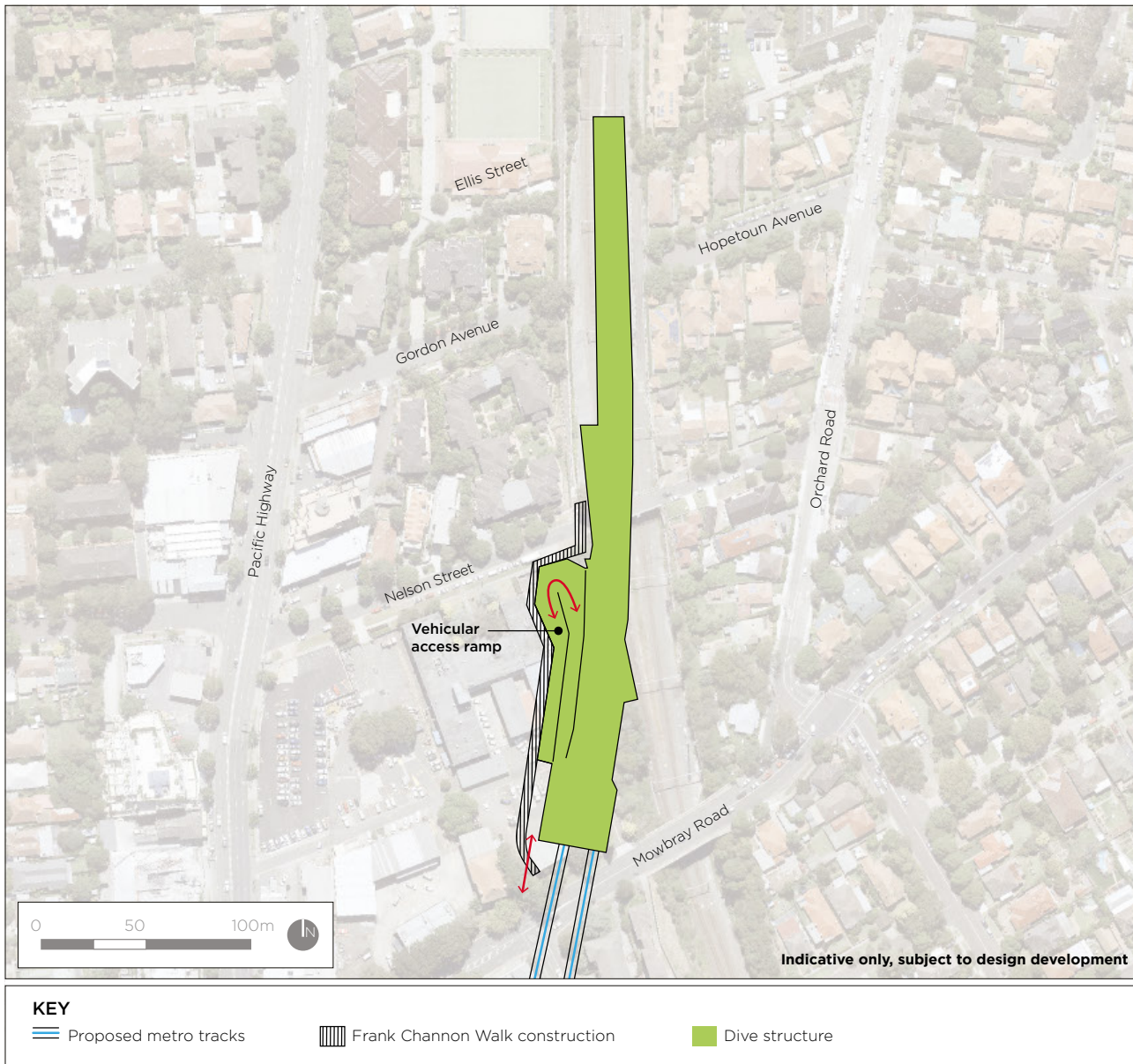
Figure 2-1 Chatswood dive structure – access for maintenance vehicles, and extension of Frank Channon Walk
