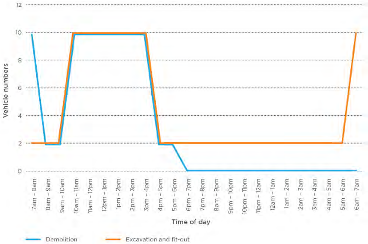
Figure 3.33 : Hourly light construction vehicle numbers (arrival only) at the Martin Place Station construction site
