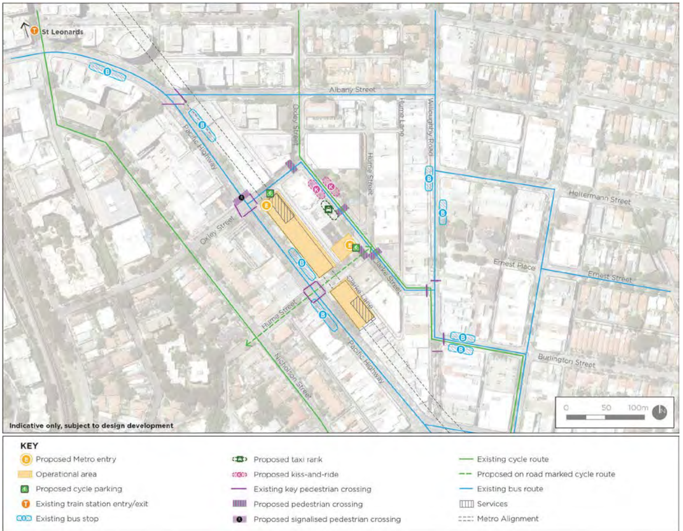
Figure 4.4 : Crows Nest Station location and transport integration
