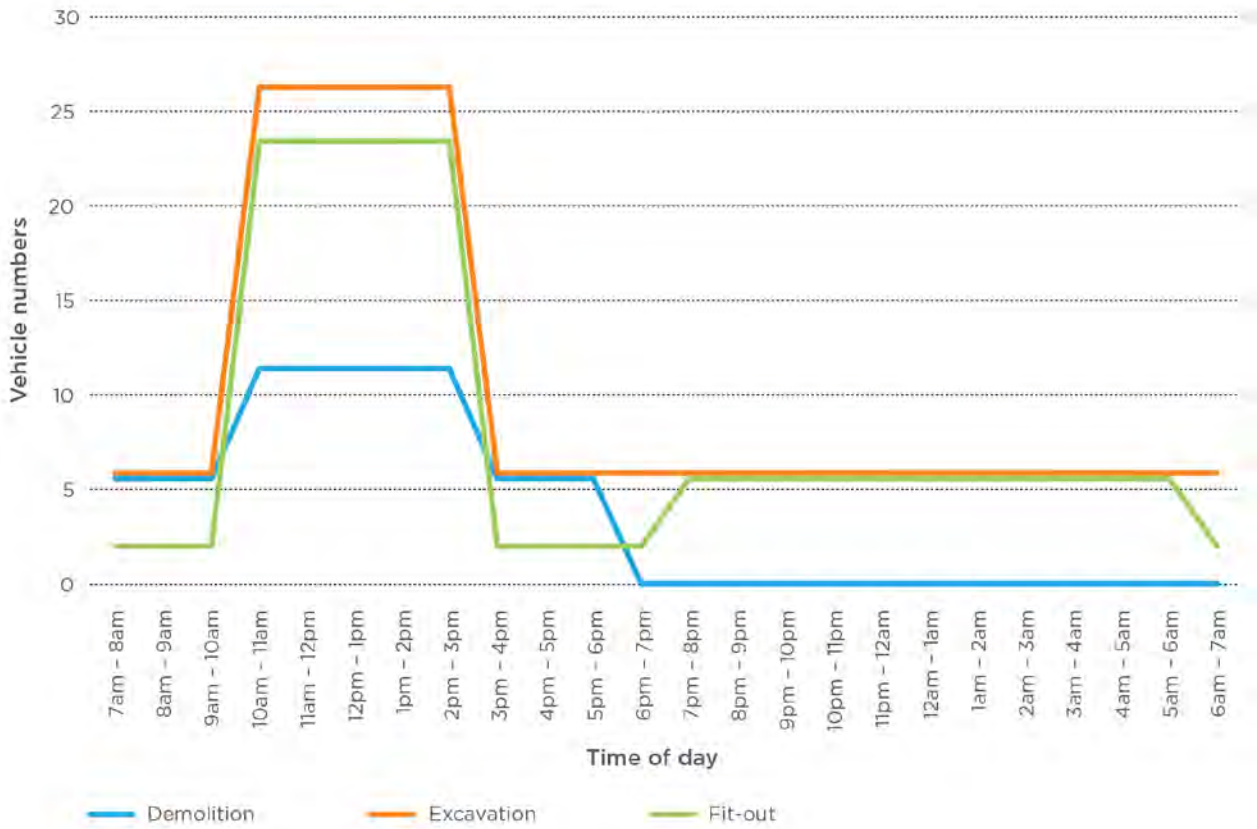
Figure 3.34 : Hourly heavy construction vehicle numbers (arrival only) at the Martin Place Station construction site
