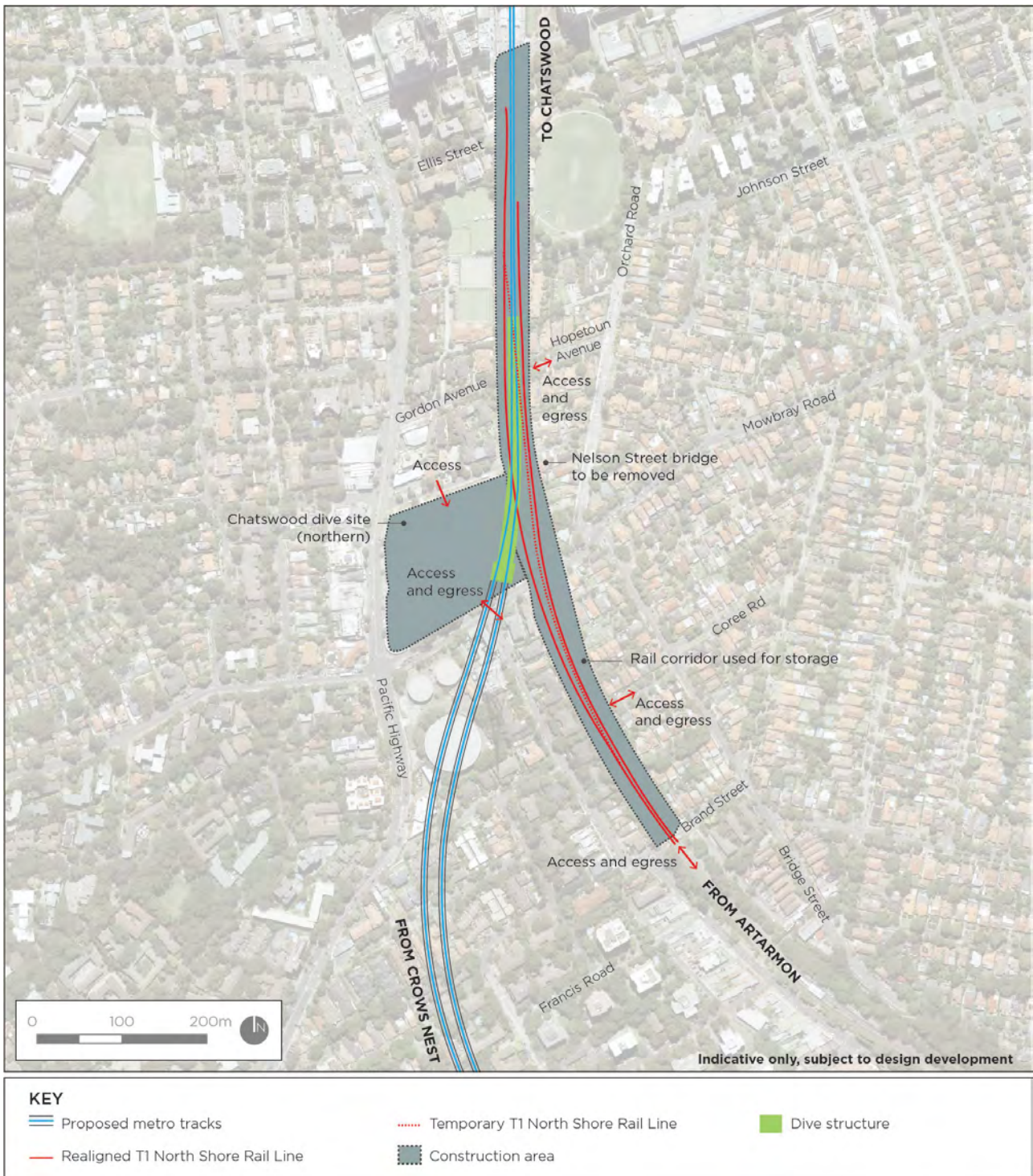
Figure 3.2: Chatswood dive site and northern surface works
