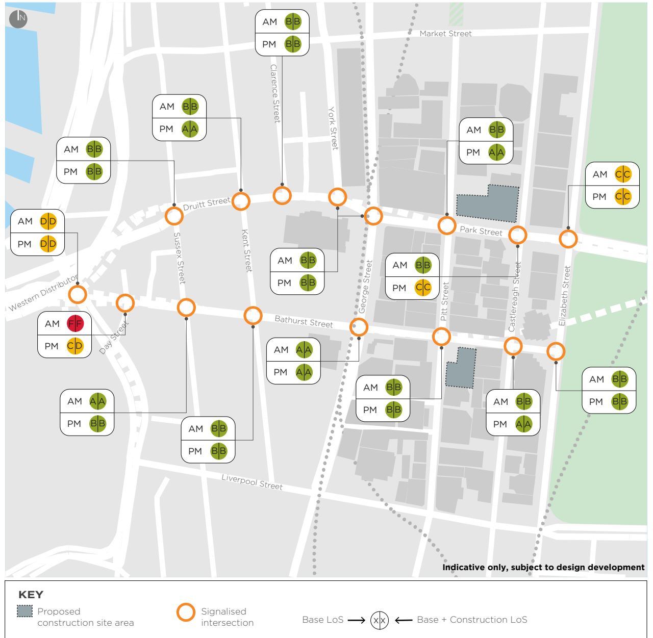
Figure 8-40 Pitt Street Station intersection performance
