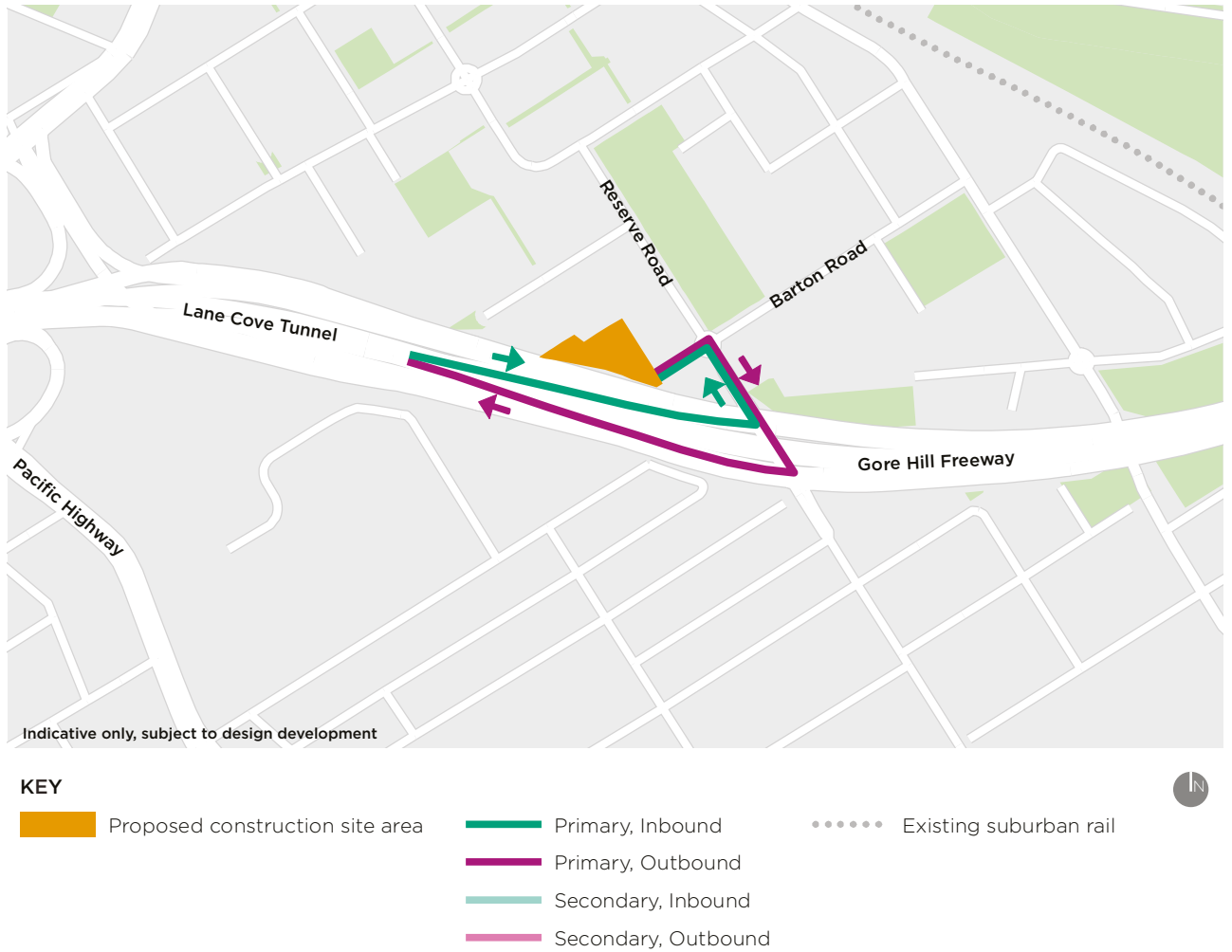
Figure 8-17 Artarmon substation construction site haul route
