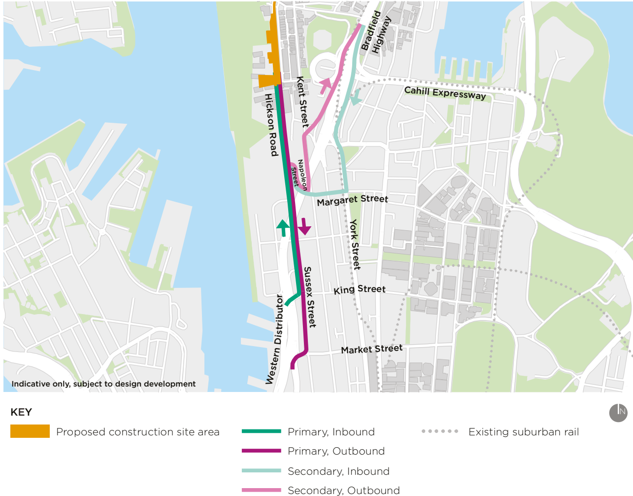
Figure 8-31 Barangaroo Station construction site haul routes
