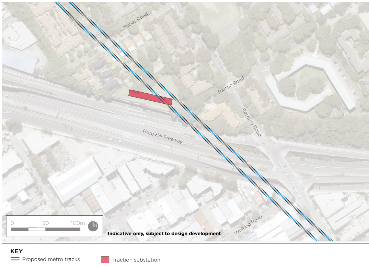
Figure 6-35 Artarmon substation - indicative plan view
