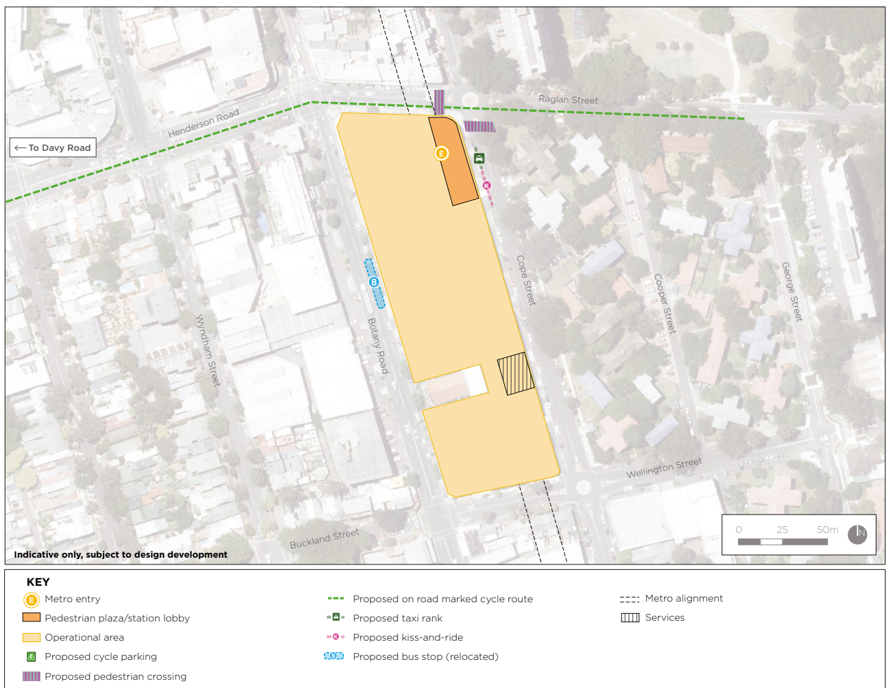
Figure 6-28 Waterloo Station – location and indicative layout
