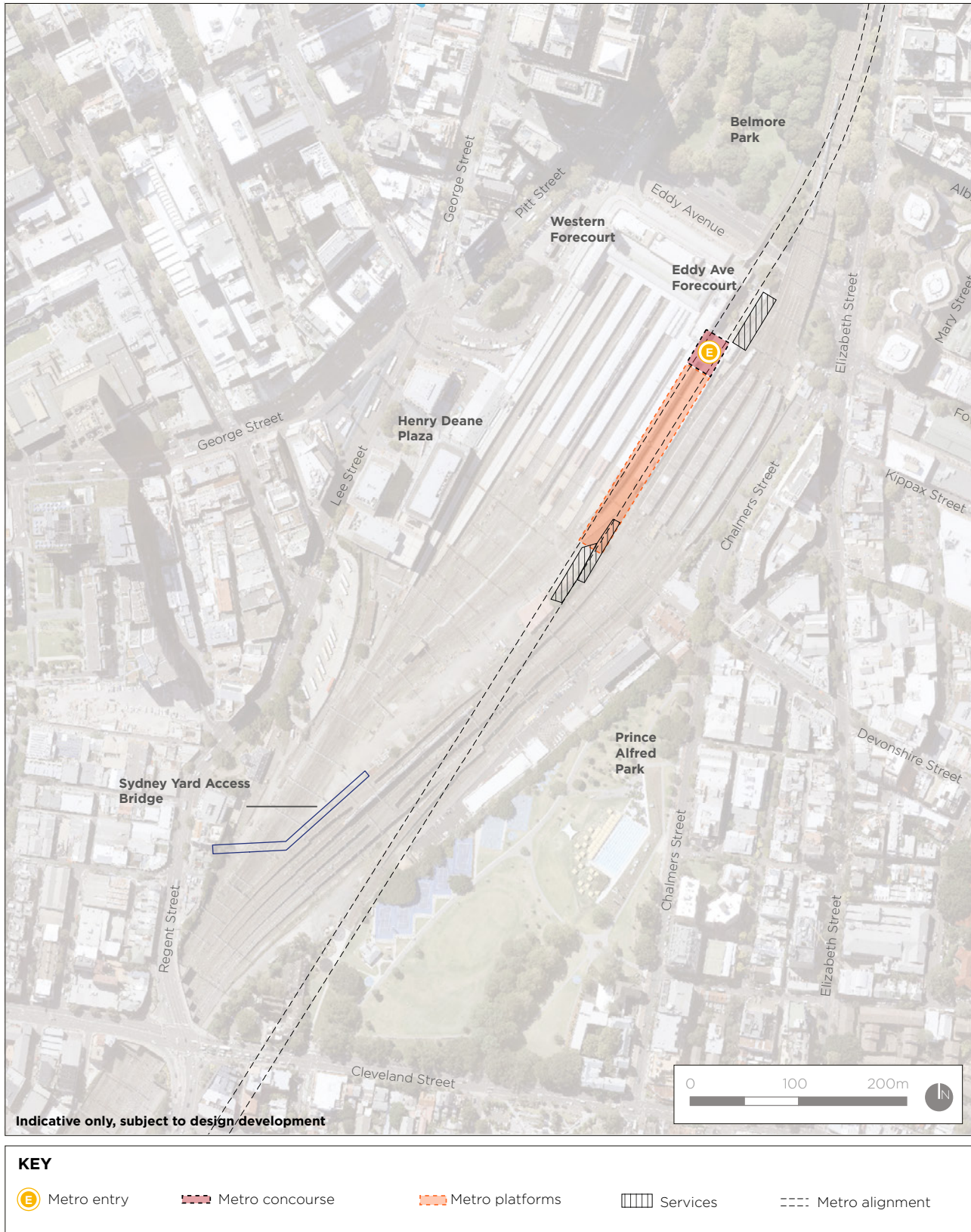
Figure 6-26 Central Station - location and indicative layout
