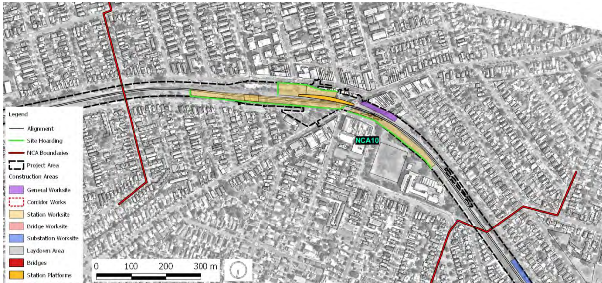
Figure 35 Punchbowl Precinct – Construction Areas
